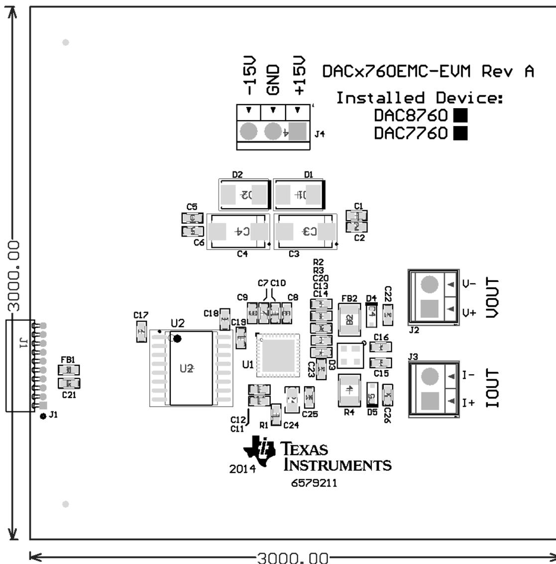
Figure 22. DACx760EMC-EVM Assembly Drawing
