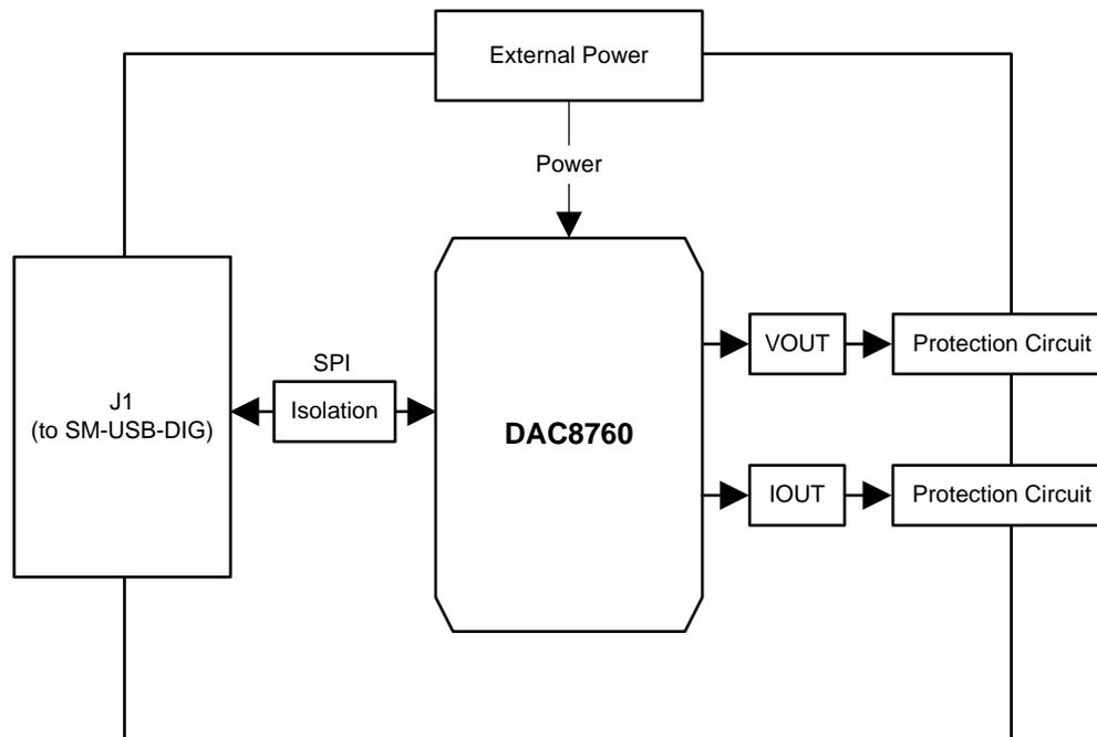
Figure 2. DAC8760EVM Block Diagram
