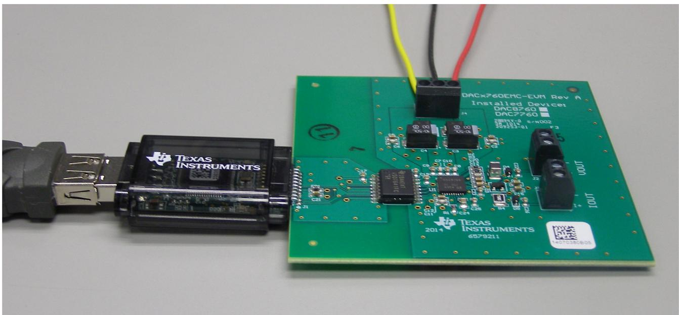
**Figure 4. SM-USB-DIG Connection to the DAC8760EVM**
