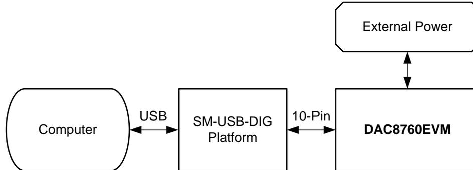
Figure 1. DAC8760EVM Hardware Setup
