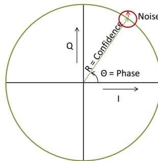
**Figure 3-7. Parametric: I and Q versus Phase**
