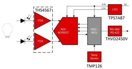
Figure 4. Optical Encoder Signal Chain
