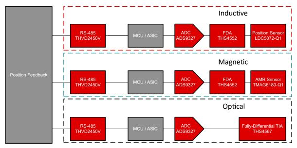
Figure 1. Encoder Signal Chain
