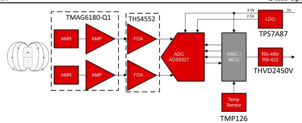
Figure 3. Magnetic Encoder Signal Chain
