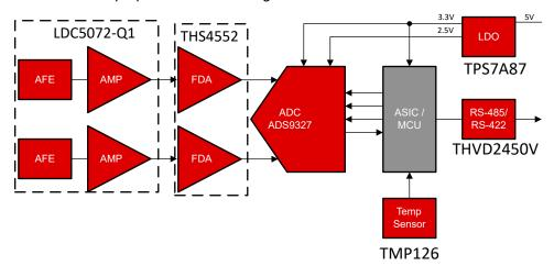
Figure 2. Inductive Encoder Signal Chain
