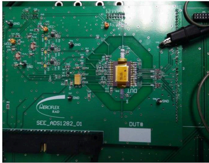
Figure 3-3. DUT Test Board
