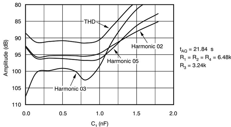
**Figure 9. THD and Harmonics as Function of Filter Capacitor  $C_1$  from [Table 2](#)**
