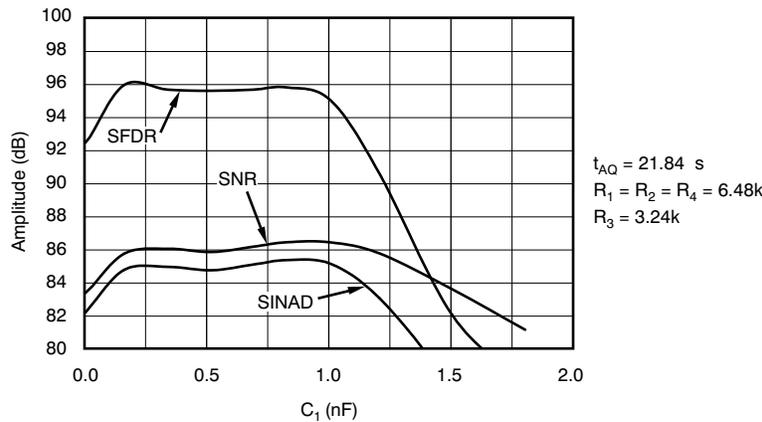
**Figure 8. AC Performance Curves as Function of Filter Capacitor  $C_1$  from [Table 2](#)**
