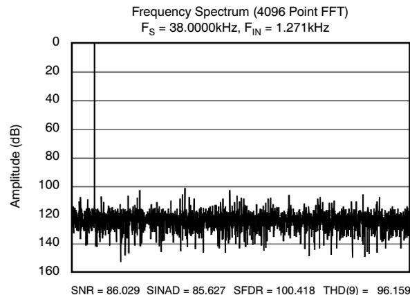
Figure 7. 4096 Point FFT of ADS8364 with Optimized Differential Input Filter Circuit from Figure 2 2
