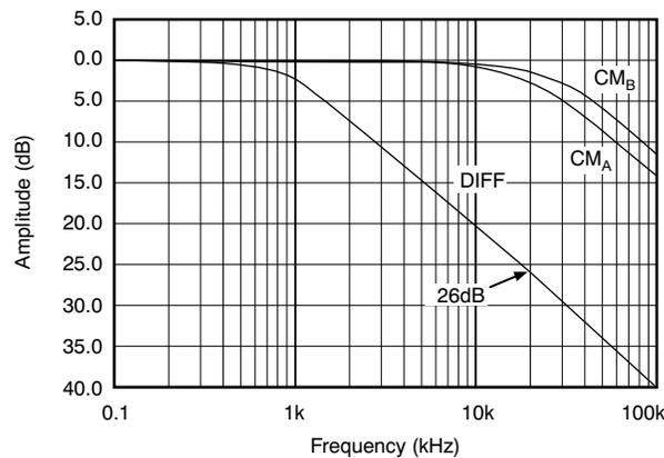
Figure 3. Frequency Response of the Equivalent Differential and Common-Mode Filters
