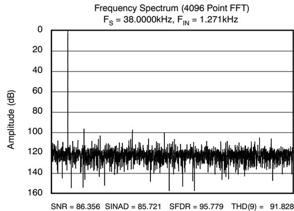
**Figure 10. 4096 Point FFT of ADS8364 with Optimized Single-Ended Input Filter Circuit from [Figure 2 2](#)**
