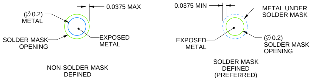
SOLDER MASK DETAILS NOT TO SCALE
