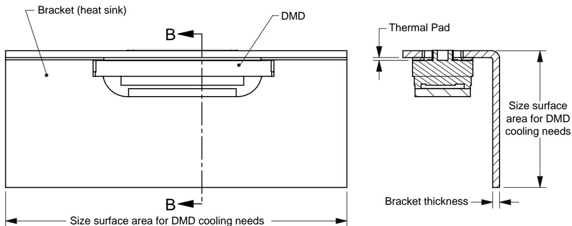
**Figure 19. Mounting Bracket Thermal Considerations**
