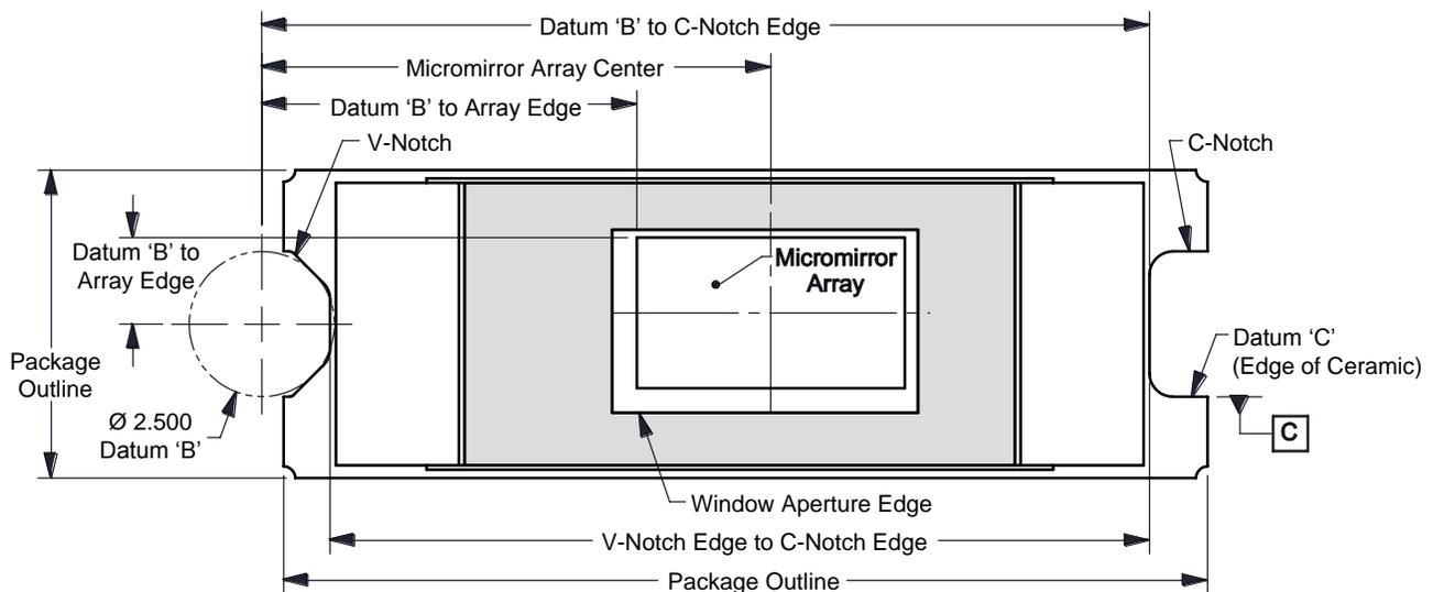
**Figure 6. Micromirror Array Location**
