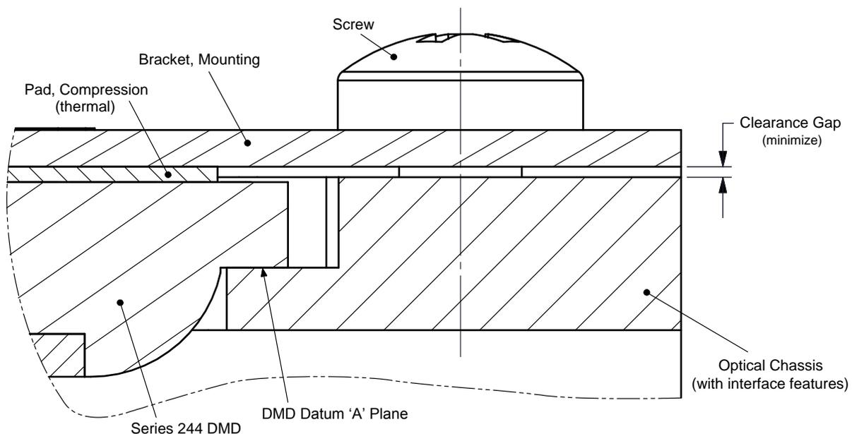
**Figure 11. Mounting Clearance Gap**
