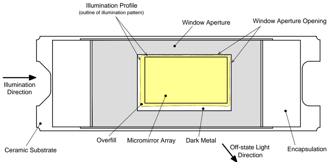
**Figure 5. Optical Illumination Overfill**
