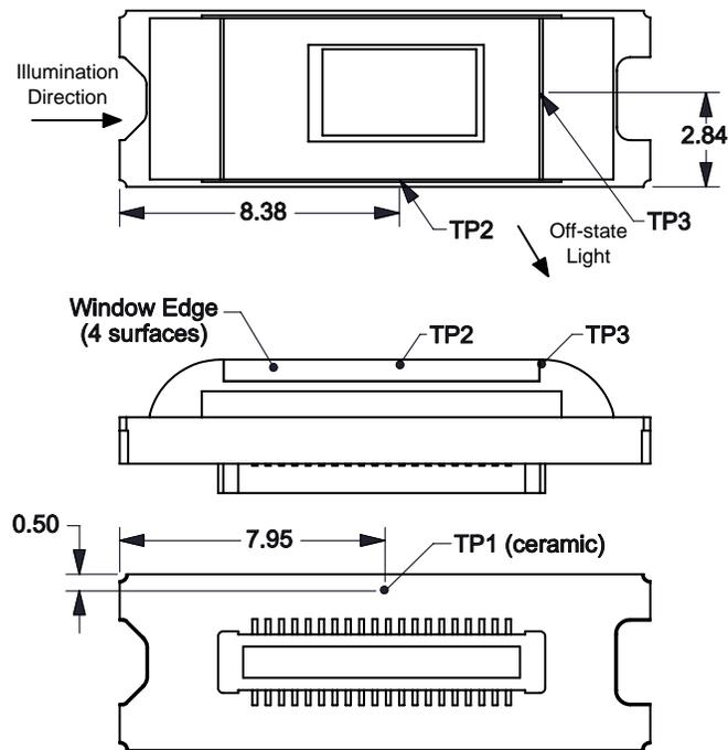
**Figure 8. Thermal Test Points**
