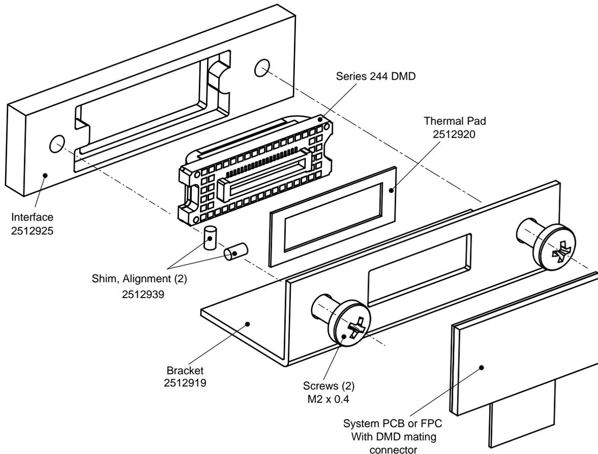
**Figure 13. Shim Alignment System Mounting Concept**
