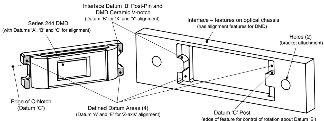
**Figure 10. Optical Interface (Alignment) Features**
