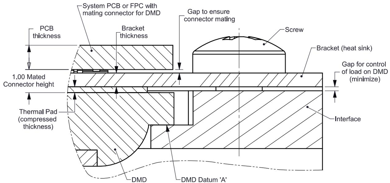
**Figure 16. Critical Gap for Control of Load**
