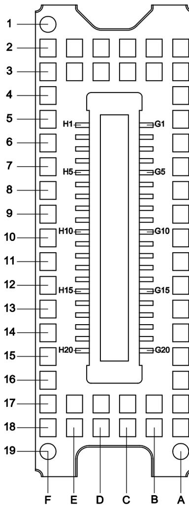
**Figure 7. Pin Numbering Scheme**
