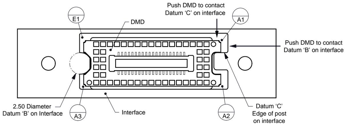
**Figure 12. Mounting Datum 'B' Contact**
