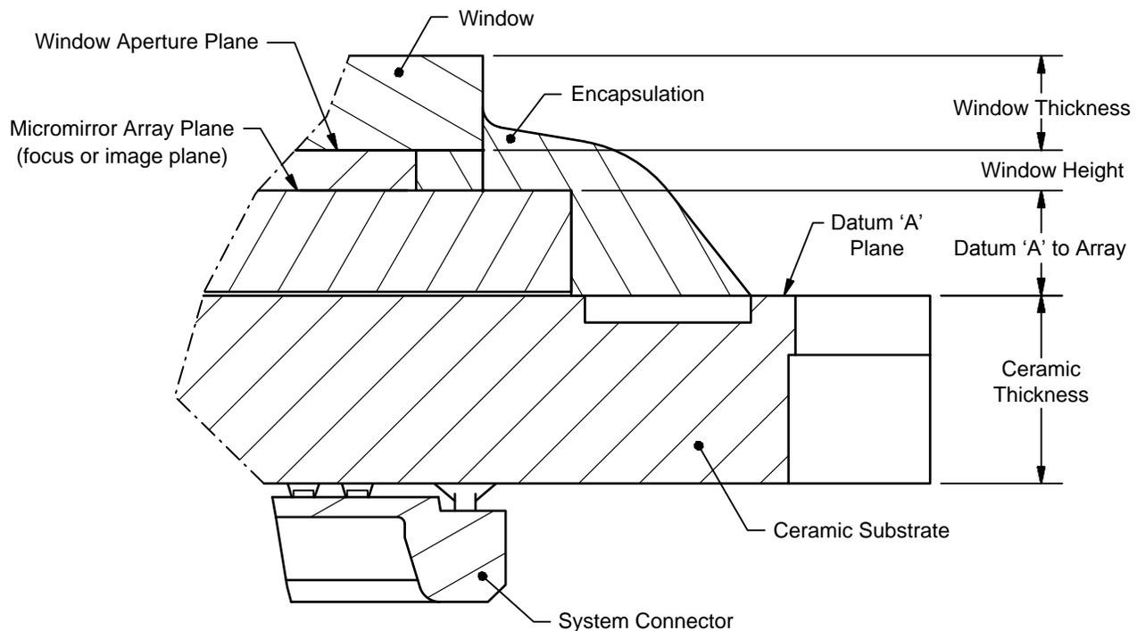
**Figure 4. DMD Cross Section View Features**
