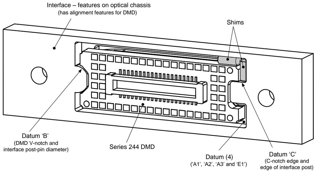
**Figure 14. Alignment Shims**
