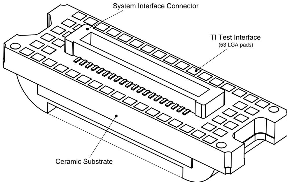
**Figure 2. DMD Features, Electrical Side**
