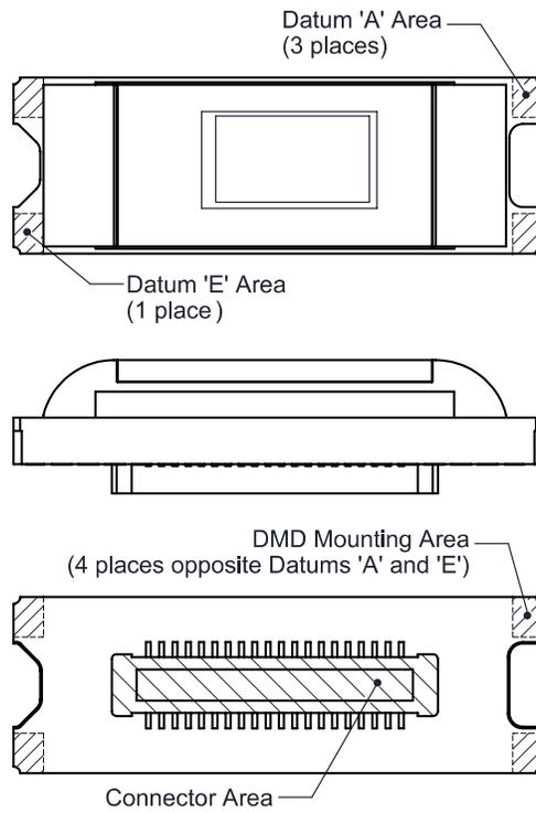
**Figure 9. DMD Mechanical Loads**
