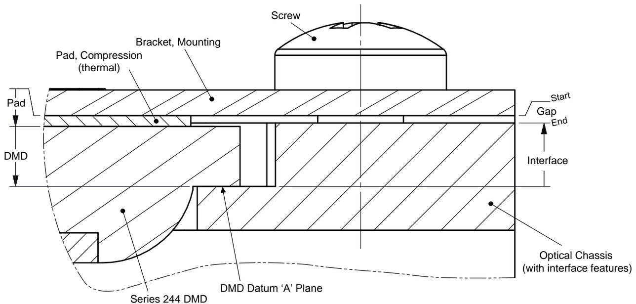
Figure 17. Gap Tolerance Analysis Schematic
