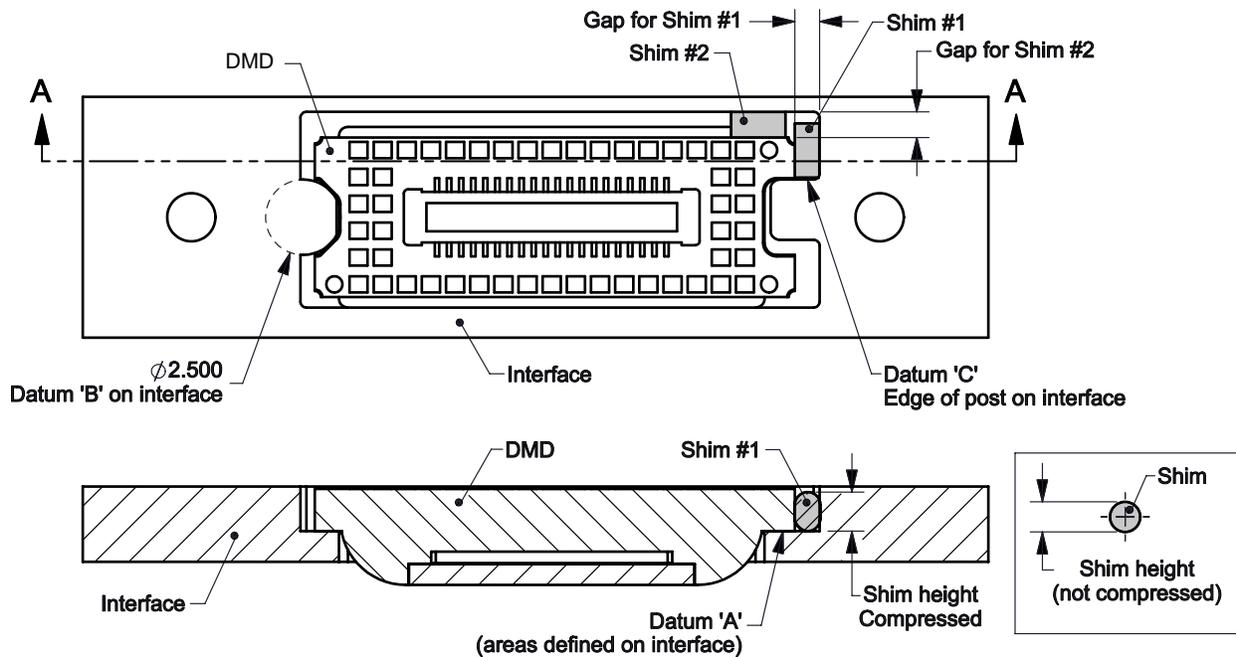
Figure 15. Gaps and Shim Shape
