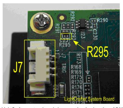
Figure 2. LightCrafter system board close-up, showing location of R295 and J7
