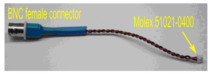
Figure 3. Adapter cable, from LightCrafter J7 to female BNC connector
