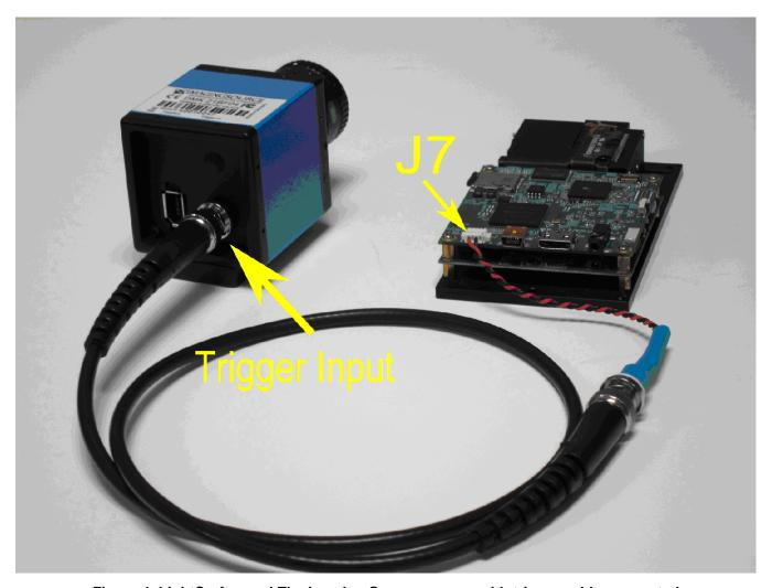
Figure 4. LightCrafter and The Imaging Source camera with trigger cable connected
