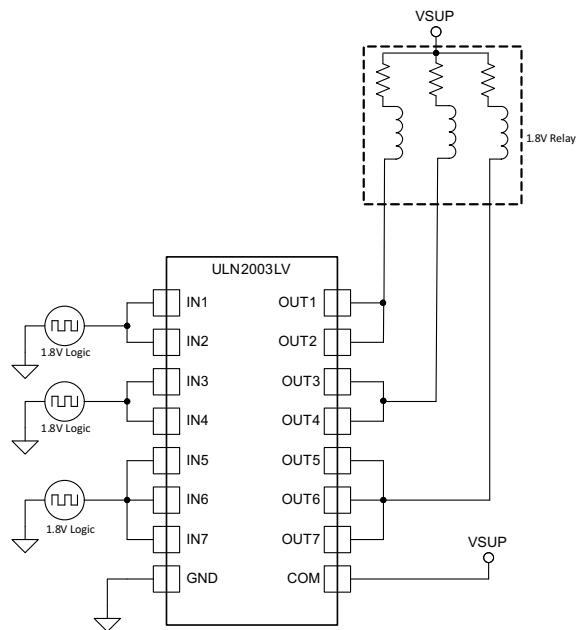
**Figure 13. ULN2003LV Driving 1.8V Relays**
