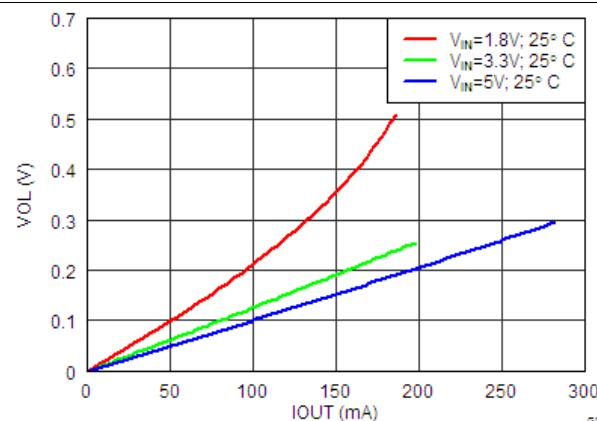
Figure 4. VOL versus IOUT 2-Channels in Parallel; VOL=0.4V
