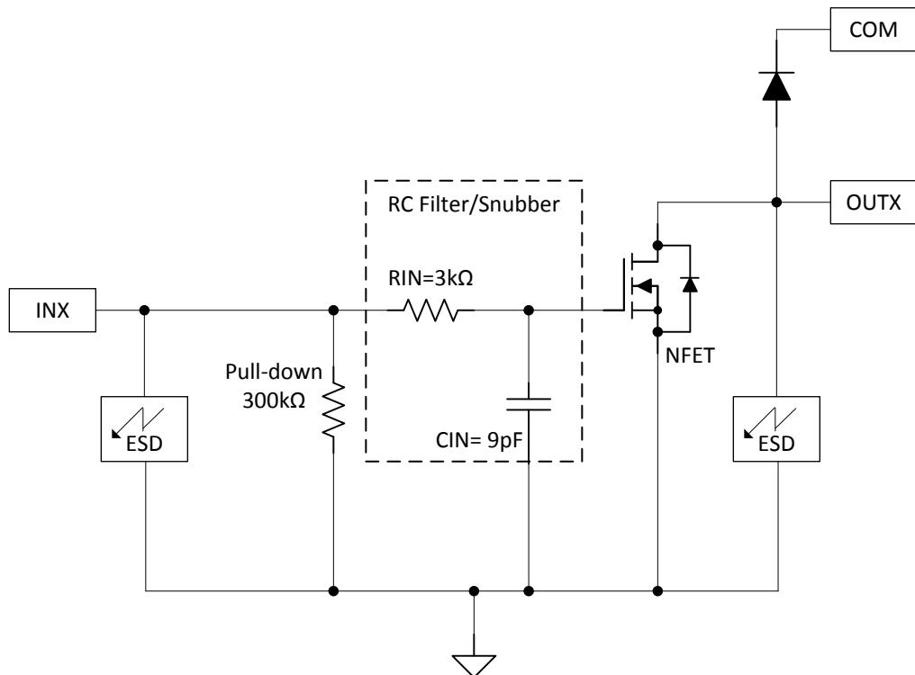
Figure 6. Channel Block Diagram
