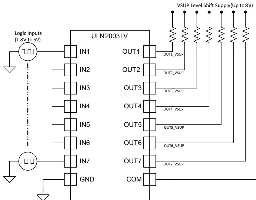
**Figure 7. ULN2003LV as Inverting Logic Level Shifter**
