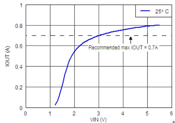
Figure 2. Load Current 7-Channels in Parallel; VOL=0.4V
