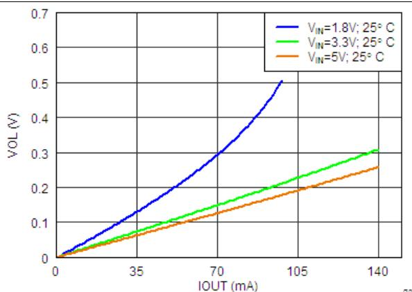
Figure 3. VOL versus IOUT  $V_{IN} = 1.8\text{V}, 3.3\text{V}, 5.0\text{V}$
