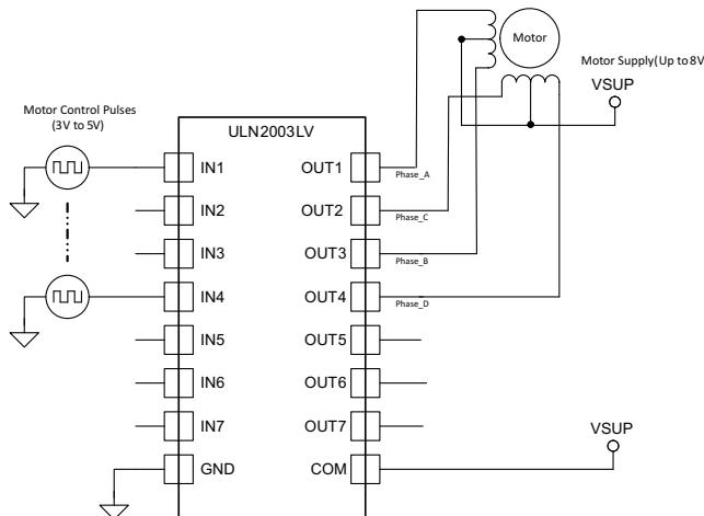
**Figure 11. ULN2003LV as a Stepper Motor Driver**
