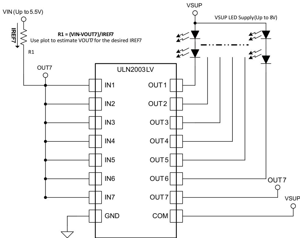
**Figure 10. ULN2003LV as a Constant Current Driver**
