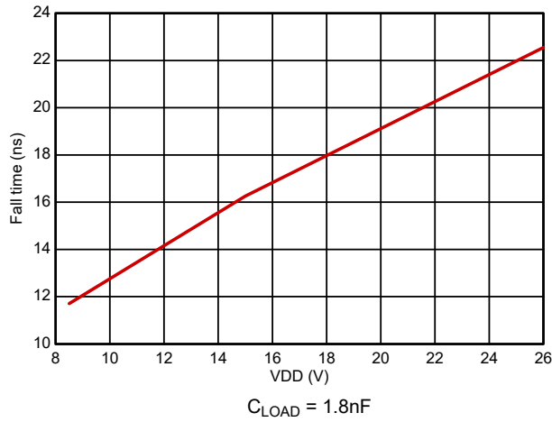
Figure 5-14. Output Fall Time
