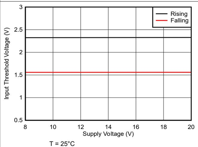
图 5-7. UCC27201A Input Threshold vs Supply Voltage
