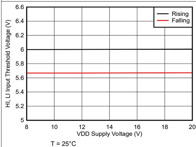
图 5-6. UCC27200A Input Threshold vs Supply Voltage
