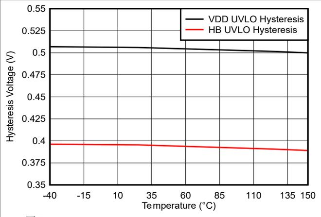
图 5-13. Undervoltage Lockout Threshold Hysteresis vs Temperature
