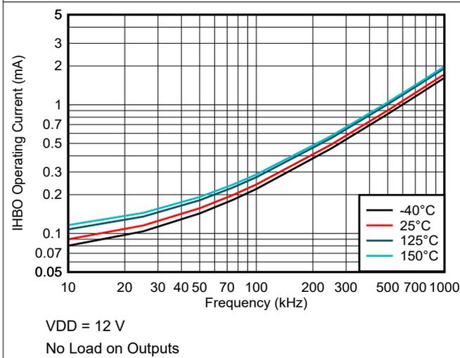
图 5-4. Boot Voltage Operating Current vs Frequency
