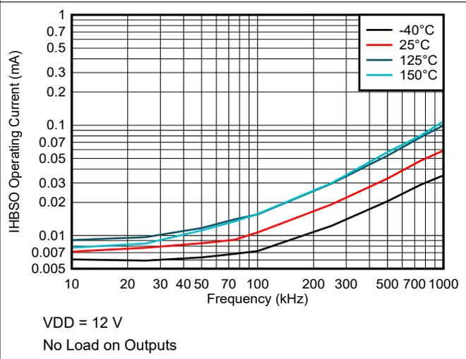
图 5-5. HB to VSS Operating Current vs Frequency
