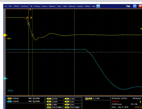
图 9-13. PWM Input (yellow) and Driver Output (blue) Falling Edge
