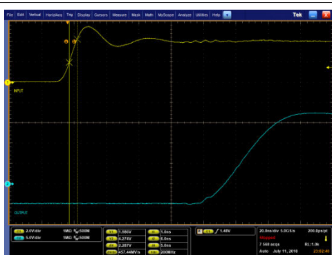
图 9-12. PWM Input (yellow) and Driver Output (blue) Rising Edge
