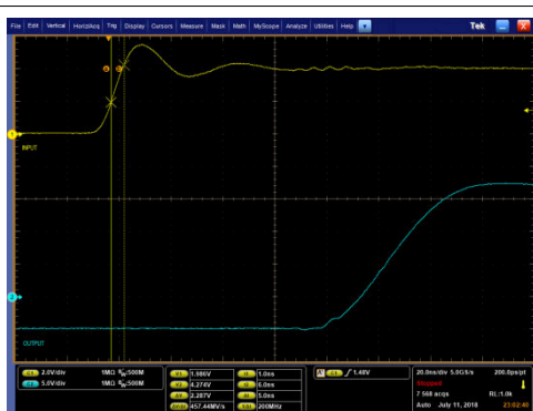
图 8-12. PWM Input (yellow) and Driver Output (blue) Rising Edge
