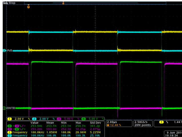
Figure 8-5. Bench Test Waveform for INA/B and OUTA/B
