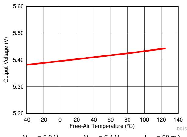
图 6-21. Isolated Supply Voltage ( $V_{ISO}$ ) vs Free-Air Temperature
