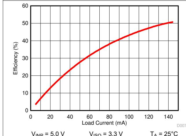
图 6-14. Power Supply Efficiency vs. Load Current ( $I_{ISO}$ )
