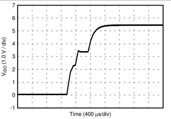
图 8-18.  $V_{ISO}$  Soft Start at 10% Rated Load, 5.0-V Input, 5.4-V Output
