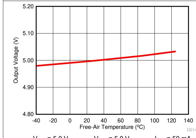
图 6-20. Isolated Supply Voltage ( $V_{ISO}$ ) vs Free-Air Temperature
