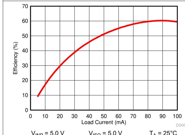
图 6-12. Power Supply Efficiency vs. Load Current ( $I_{ISO}$ )
