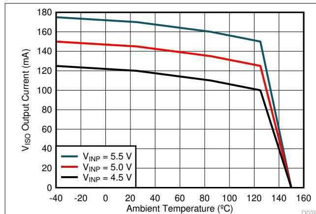
图 6-10. Maximum  $V_{ISO}$  Output Current vs. Temperature
