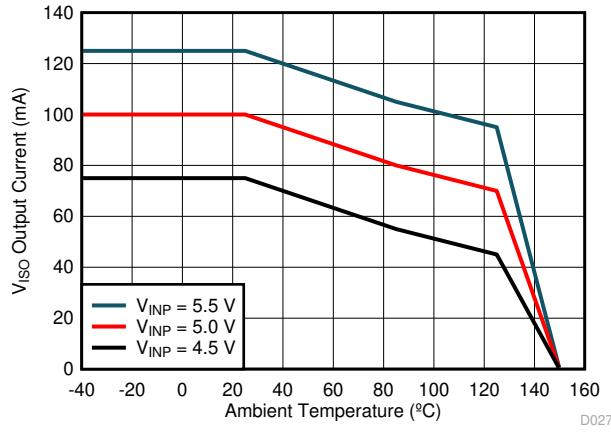
$V_{ISO} = 5.4 \text{ V}$ 图 6-9. Maximum  $V_{ISO}$  Output Current vs. Temperature
