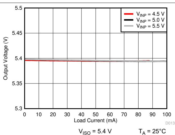
图 6-17. Isolated Supply Voltage ( $V_{ISO}$ ) vs Load Current ( $I_{ISO}$ )
