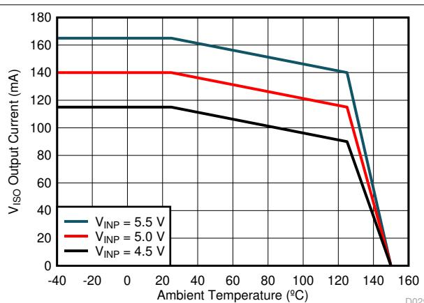
图 6-11. Maximum  $V_{ISO}$  Output Current vs. Temperature
