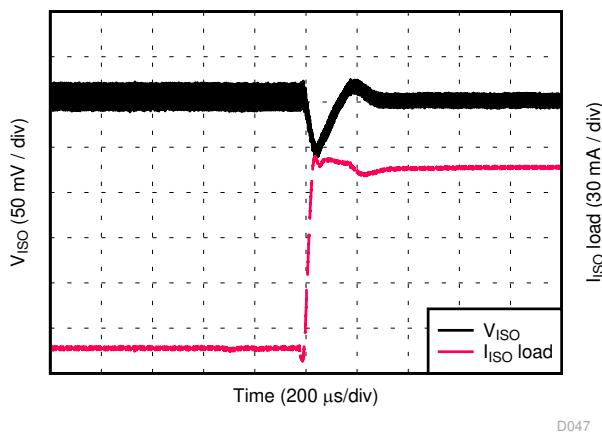
图 8-17.  $V_{ISO}$  Load Transient Response, 90% to 10% Load Step, 5.0-V Input, 3.3-V Output
