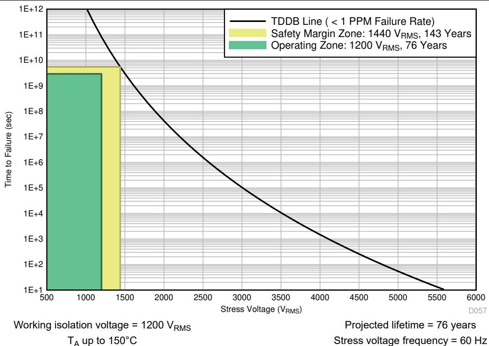
图 6-1. Insulation Lifetime Projection Data
