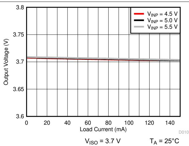
图 6-19. Isolated Supply Voltage ( $V_{ISO}$ ) vs Load Current ( $I_{ISO}$ )
