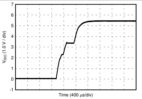
图 8-19.  $V_{ISO}$  Soft Start at 90% Rated Load, 5.0-V Input, 5.4-V Output
