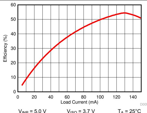
图 6-15. Power Supply Efficiency vs. Load Current ( $I_{ISO}$ )
