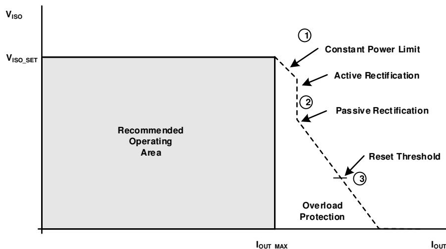
图 7-1.  $V_{ISO}$  Load Recommended Operating Area Description
