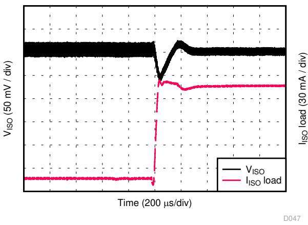
图 8-16.  $V_{ISO}$  Load Transient Response, 10% to 90% Load Step, 5.0-V Input, 3.3-V Output
