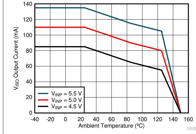
$V_{ISO} = 5.0 \text{ V}$ 图 6-8. Maximum  $V_{ISO}$  Output Current vs. Temperature
