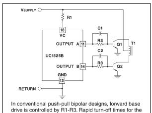
power devices are acheived with speed-up capacitors C,
