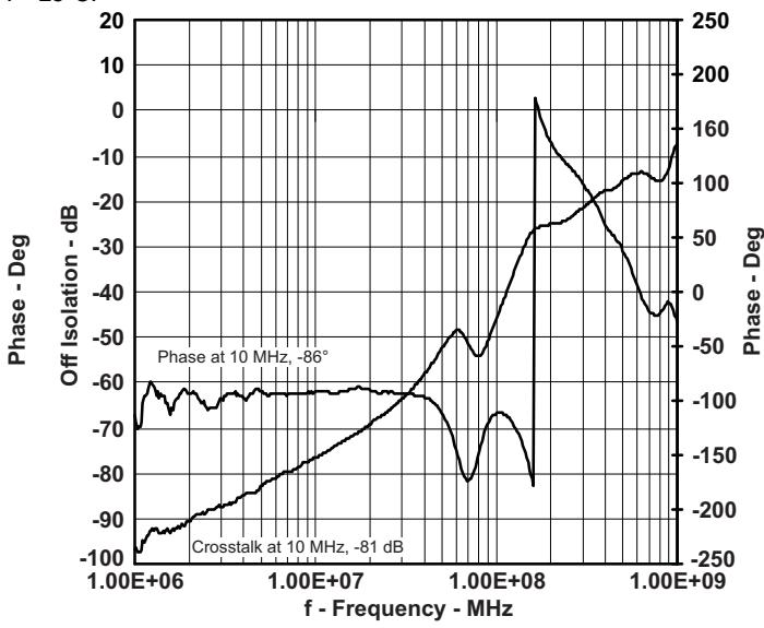
Figure 4. Non-adjacent Crosstalk vs Frequency
