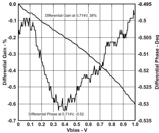
Figure 6. Differential Phase/Gain vs Vbias
