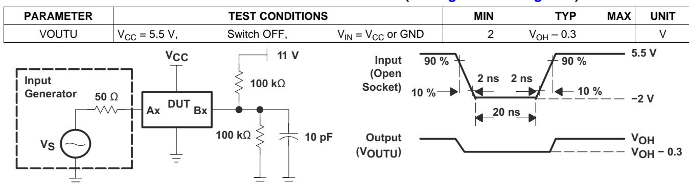
**Figure 7. Device Test Setup**
