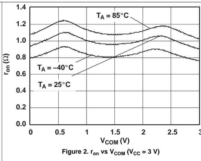
Figure 2.  $r_{on}$  vs  $V_{COM}$  ( $V_{CC} = 3\text{ V}$ )
