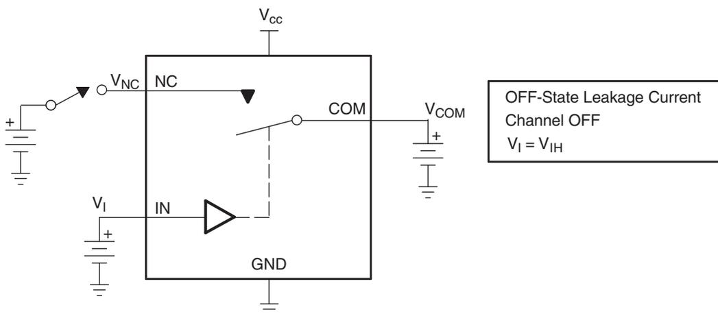
Figure 14. OFF-State Leakage Current ( $I_{COM(OFF)}$ ,  $I_{NC(OFF)}$ ,  $I_{COM(PWROFF)}$ ,  $I_{NC(PWROFF)}$ )
