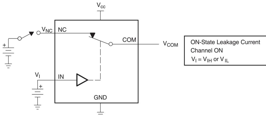
Figure 15. ON-State Leakage Current ( $I_{COM(ON)}$ ,  $I_{NC(ON)}$ )
