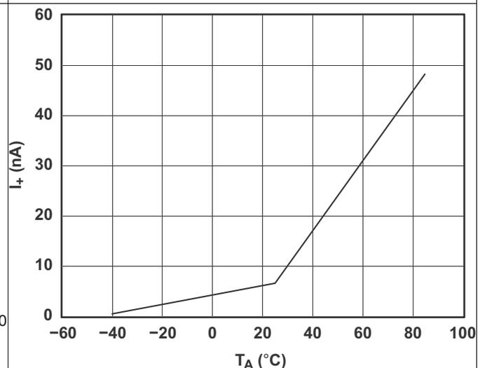
Figure 12. Power-Supply Current vs Temperature ( $V_{CC} = 5\text{ V}$ )
