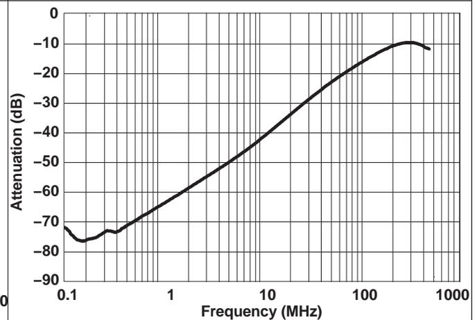
Figure 10. OFF Isolation vs Frequency ( $V_{CC} = 5\text{ V}$ )
