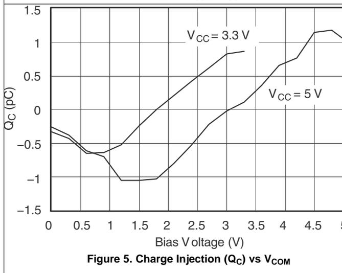
Figure 5. Charge Injection ( $Q_C$ ) vs  $V_{COM}$
