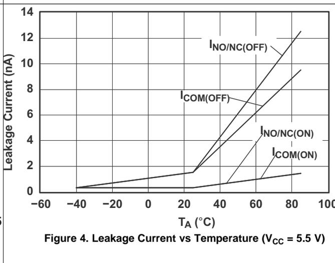
Figure 4. Leakage Current vs Temperature ( $V_{CC} = 5.5\text{ V}$ )
