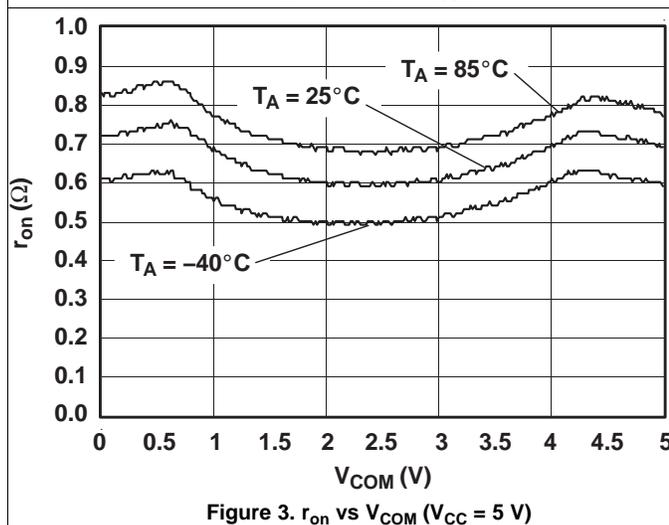
Figure 3.  $r_{on}$  vs  $V_{COM}$  ( $V_{CC} = 5\text{ V}$ )
