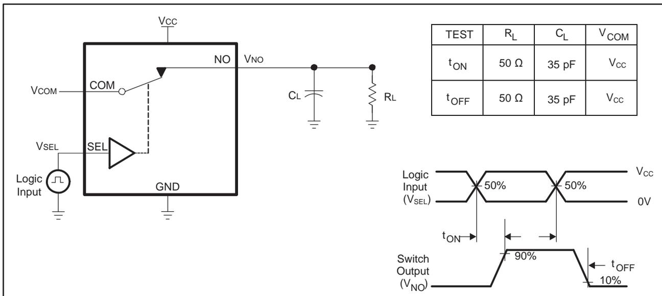
Figure 8. Turn-On ( $t_{ON}$ ) and Turn-Off Time ( $t_{OFF}$ )
