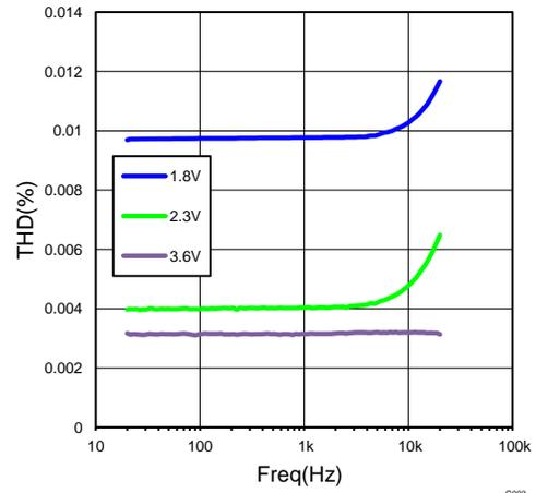
Figure 6. Total Harmonic Distortion
