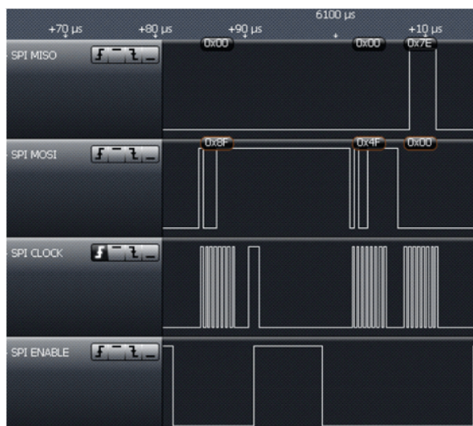
Figure 6-25. Reset FIFO and Read RSSI
