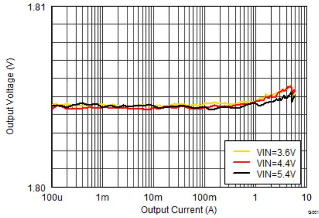
图 16. Output Voltage vs Output Current (Load Regulation)
