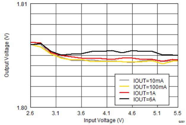
图 17. Output Voltage vs Input Voltage (Line Regulation)
