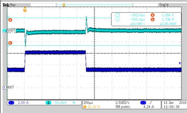
图 32. Load Transient Response (PWM-PWM), Load Step 3 to 6 A
