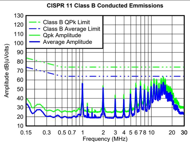
$V_{IN} = 24V$        $V_{OUT} = 5V$        $f_{SW} = 1MHz$
