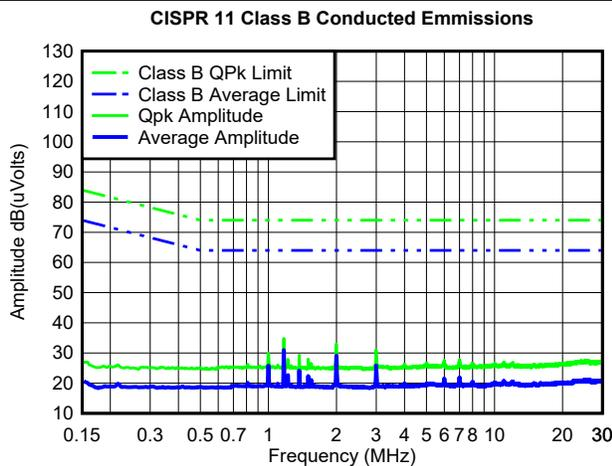
$V_{IN} = 24V$        $V_{OUT} = 5V$        $f_{SW} = 1MHz$
