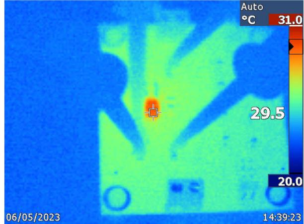
$V_{IN} = 24V$      $V_{OUT} = 5V$     150mA, 1MHz
