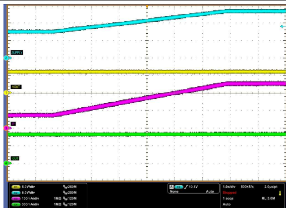
Ch. 1 = V_{(SUPPLY)} Ch. 2 = V_{(OUT)} Ch. 3 = I_{(P)} Ch. 4 = I_{(LED)} V_{(SUPPLY)} increases from 9 V to 16 V
