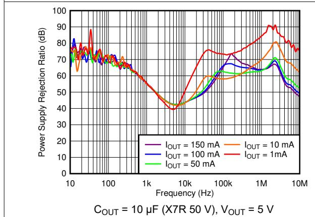
图 5-9. PSRR vs Frequency and  $I_{OUT}$
