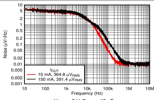
图 5-12. Noise vs Frequency at 5.0 V
