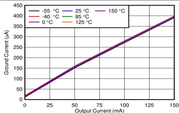
图 5-24. Ground Current ( $I_{GND}$ ) vs  $I_{OUT}$
