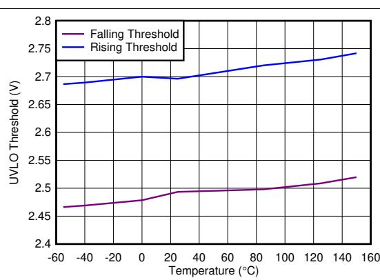
图 5-28. Undervoltage Lockout (UVLO) Threshold vs Temperature
