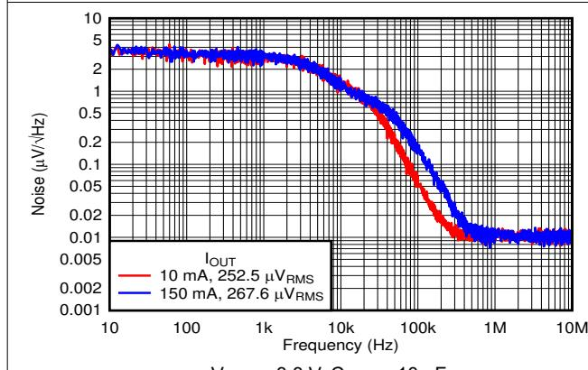
图 5-11. Noise vs Frequency at 3.3 V
