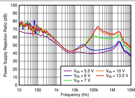
图 5-10. PSRR vs Frequency and  $V_{IN}$
