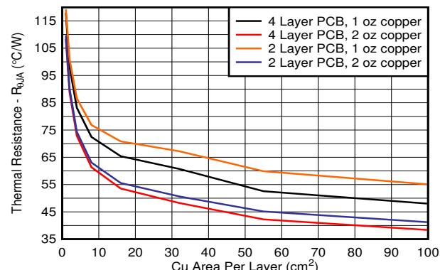
图 7-4.  $R_{\theta JA}$  vs Copper Area 2s2p DCY Package
