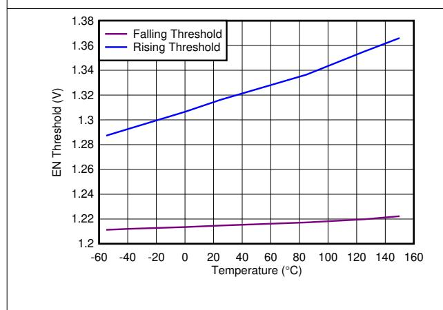
图 5-27. EN Threshold vs Temperature
