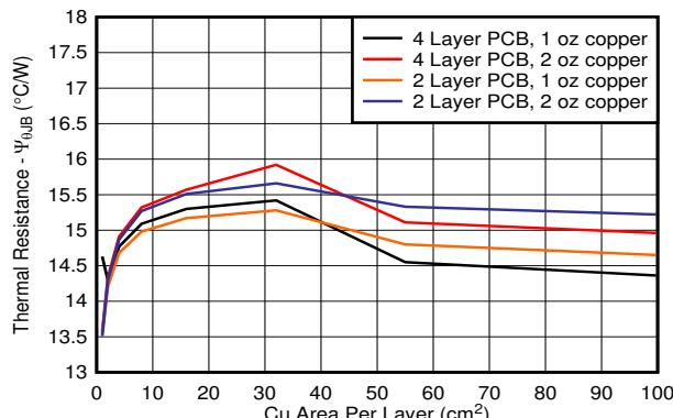
图 7-5.  $\psi_{JB}$  vs Copper Area 2s2p DCY Package
