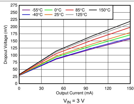
图 5-8. Dropout Voltage ( $V_{DO}$ ) vs  $I_{OUT}$
