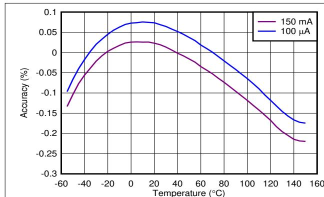
图 5-1. Accuracy vs Temperature
