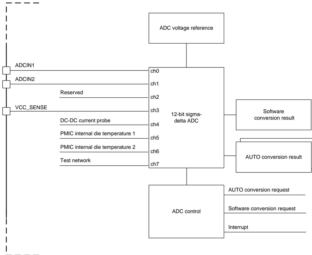
图 5-15. Block Diagram of the GPADC
