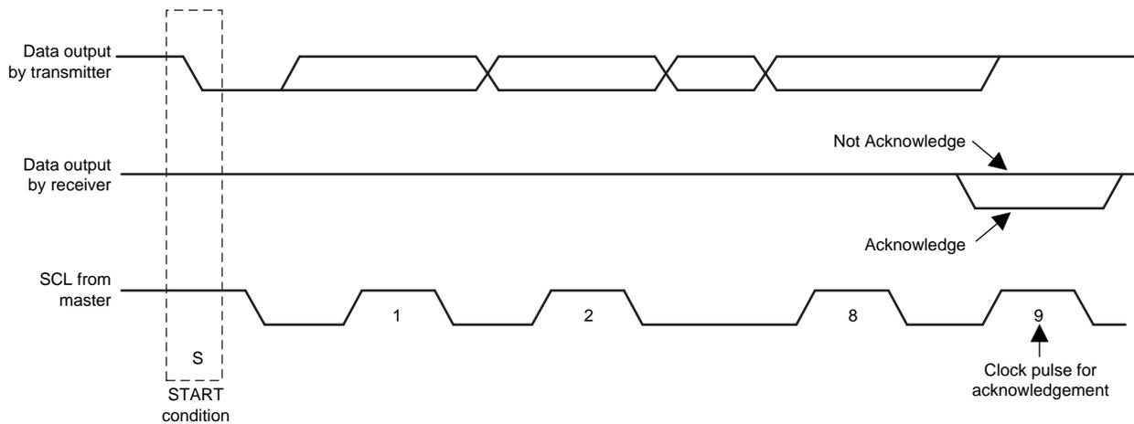
图 5-19. Acknowledge on the I<sup>2</sup>C Bus
