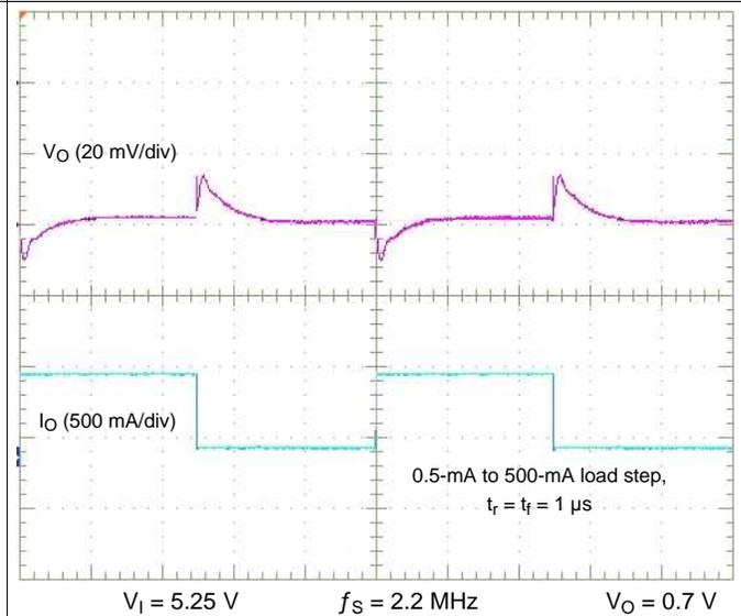
图 6-8. Typical SMPS Load Transient Response for SMPS4
