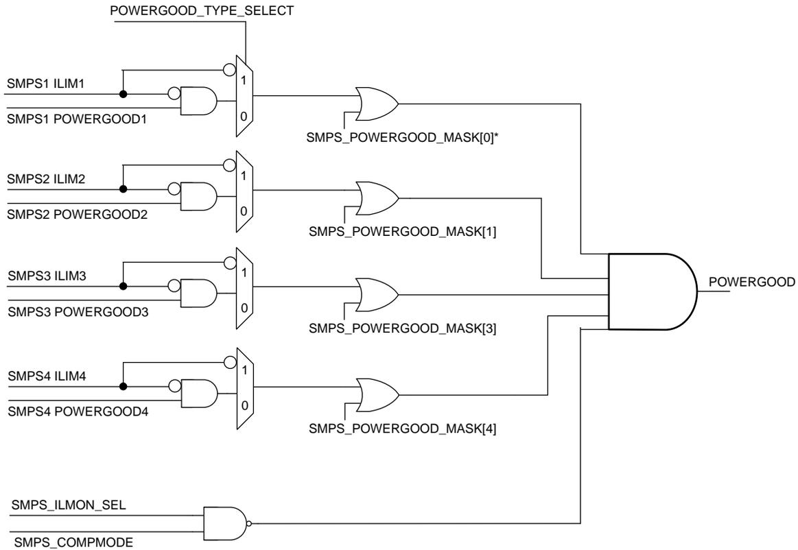
\*When operating in dual phase, SMPS\_POWERGOOD\_MASK[0] controls the monitoring of SMPS12.
