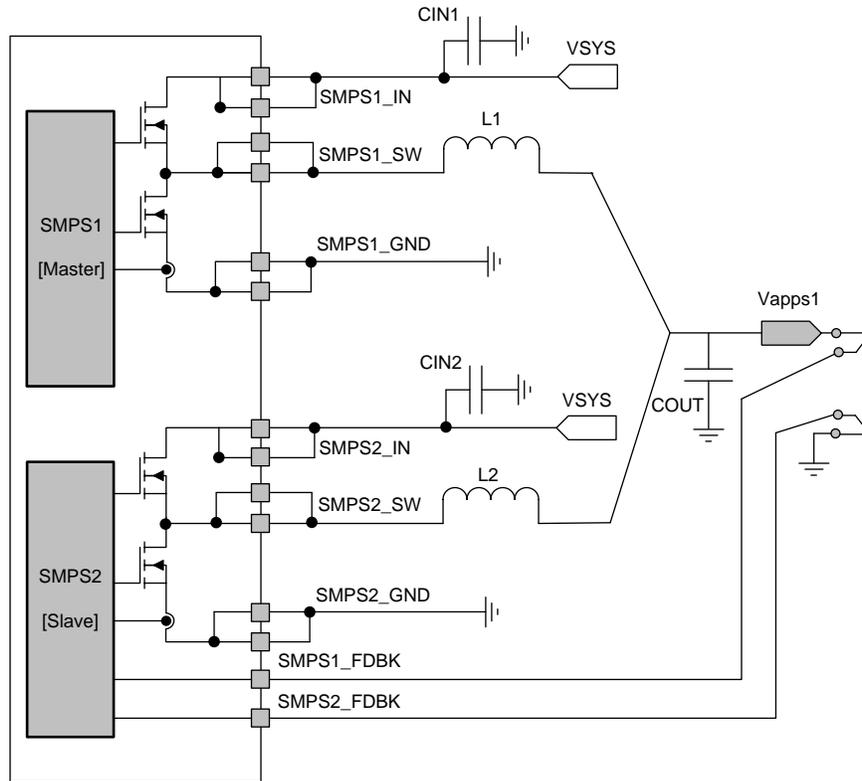
图 5-14. SMPS1&2 Dual-Phase Configuration
