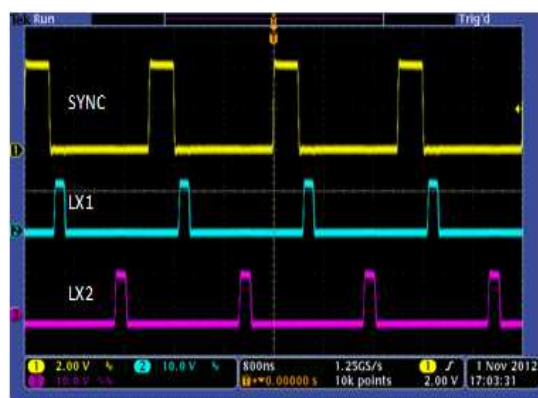
Figure 32. Synchronization at 500 kHz
