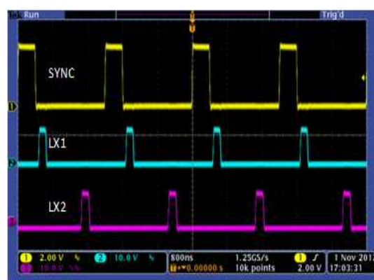
Figure 31. Synchronization at 500 kHz
