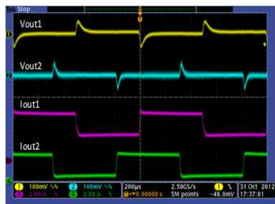
Figure 24. Load Transient, Buck 1 2.5 A - 4.5 A, Buck2 0.5 A - 2.5 A
