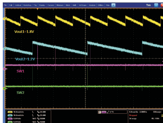
Figure 12. Buck 1 and Buck 2 in PSM Mode
