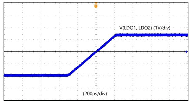
$V_{IN} = 5.0V$        $V_{OUT} = 3.3V$        $T_A = 25^\circ C$
