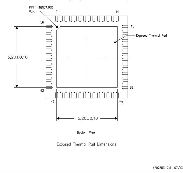
NOTE: All linear dimensions are in millimeters
