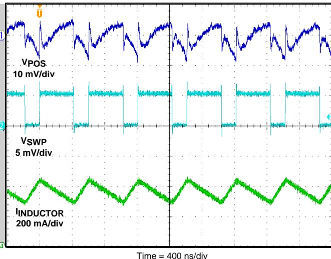
**Figure 6. SWITCH PIN, INDUCTOR CURRENT and OUTPUT V<sub>POS</sub> BOOST, V<sub>POS</sub> = 5 V, I<sub>OUT</sub> = 250 mA**
