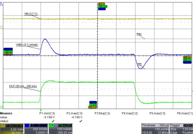
**Figure 10. V<sub>NEG</sub> LOAD TRANSIENT**
