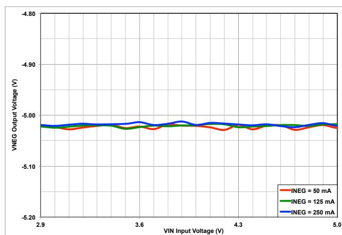
Figure 3.  $V_{NEG}$  OUTPUT VOLTAGE vs. INPUT VOLTAGE
