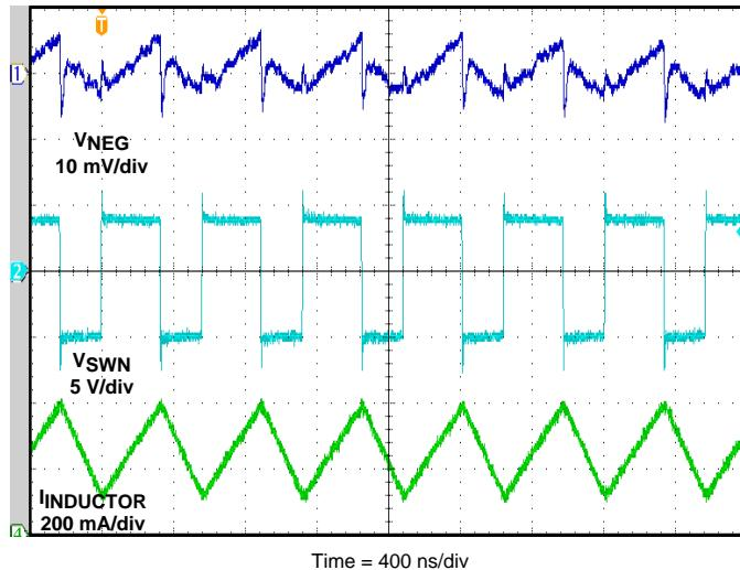
**Figure 7. SWITCH PIN, INDUCTOR CURRENT and OUTPUT V<sub>NEG</sub> BOOST, V<sub>NEG</sub> = -5 V, I<sub>OUT</sub> = 100 mA**
