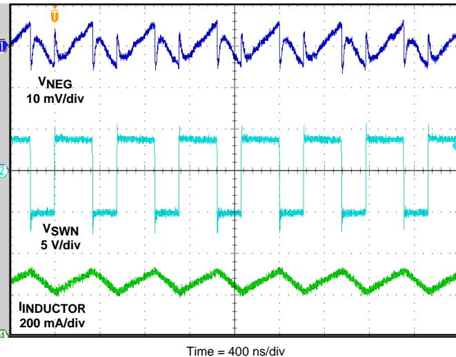
**Figure 8. SWITCH PIN, INDUCTOR CURRENT and OUTPUT V<sub>NEG</sub> BOOST, V<sub>NEG</sub> = -5 V, I<sub>OUT</sub> = 250 mA**
