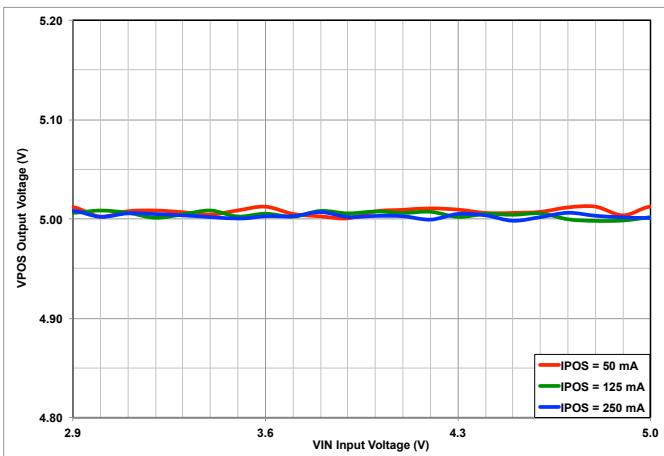
Figure 2.  $V_{POS}$  OUTPUT VOLTAGE vs. INPUT VOLTAGE
