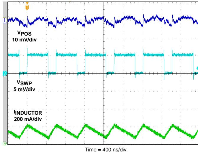
**Figure 5. SWITCH PIN, INDUCTOR CURRENT and OUTPUT V<sub>POS</sub> BOOST, V<sub>POS</sub> = 5 V, I<sub>OUT</sub> = 100 mA**
