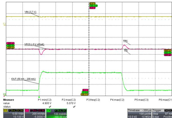
**Figure 9. V<sub>POS</sub> LOAD TRANSIENT**
