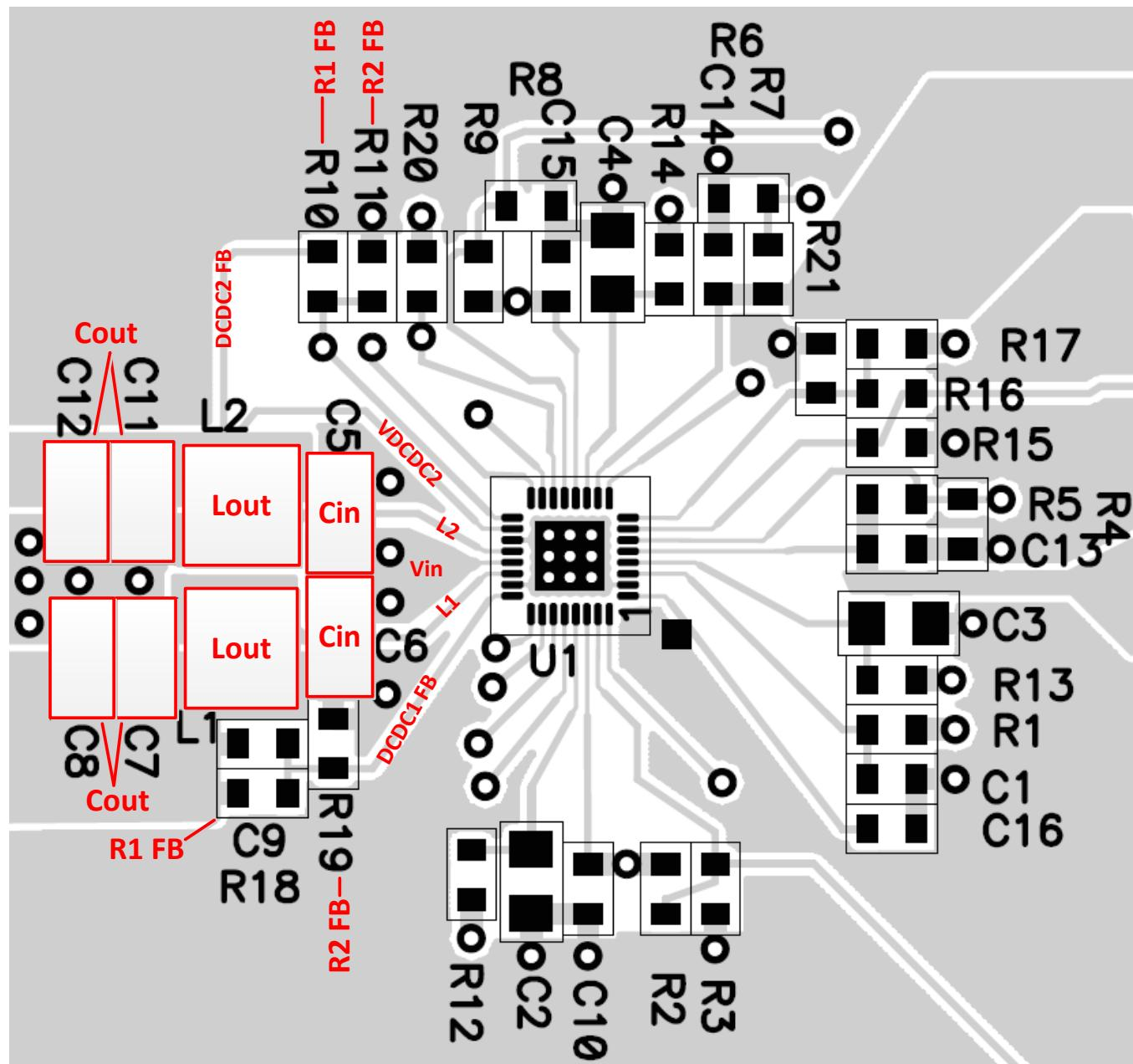
Figure 25. Layout Example from EVM for TPS65051-Q1
