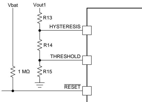
Figure 11. **RESET** Circuit
