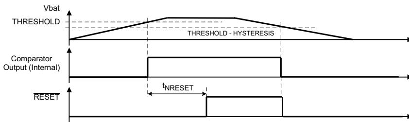
**Figure 8. RESET Pulse Circuit**
