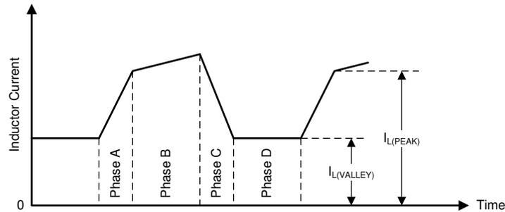
**图 7-2. Inductor Current Waveform when  $V_I > V_O$  (CCM)**
