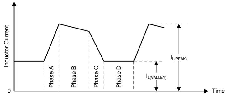
**图 7-4. Inductor Current Waveform when  $V_I < V_O$  (CCM)**
