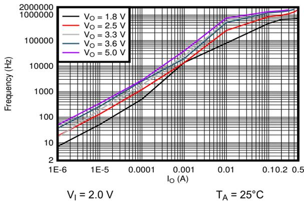
图 8-4. Typical Burst Switching Frequency versus Output Current
