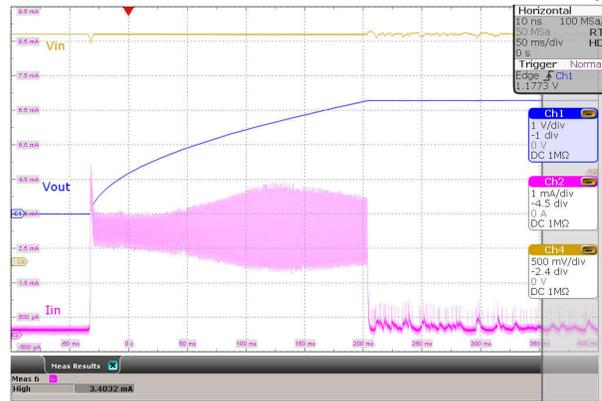
$V_I = 3.3\text{ V}, V_O = 3.3\text{ V}$        $C_1 = 32\ \mu\text{F}, C_O = 300\ \mu\text{F}$
