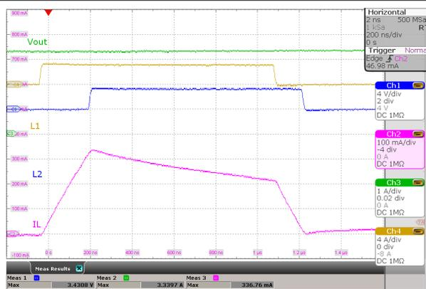
图 8-12. Switching Waveforms, Buck-Boost Operation
