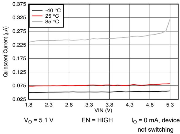
**图 6-1. Quiescent Current into VIN versus Input Voltage**
