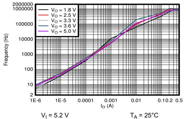
图 8-5. Typical Burst Switching Frequency versus Output Current
