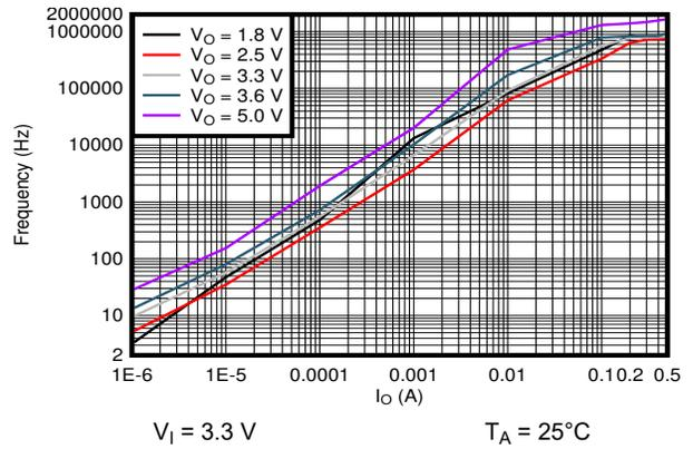
图 8-3. Typical Burst Switching Frequency versus Output Current
