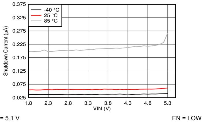
**图 6-3. Shutdown Current versus Input Voltage**
