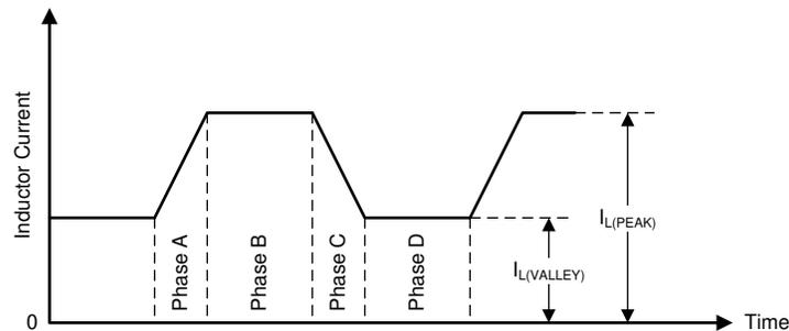
**图 7-3. Inductor Current Waveform when  $V_I = V_O$  (CCM)**
