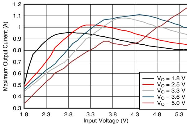
图 8-2. Typical Output Current Capability versus Input Voltage
