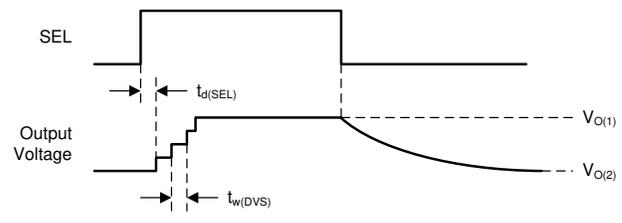
图 7-11. Dynamic Voltage Scaling with Light Load
