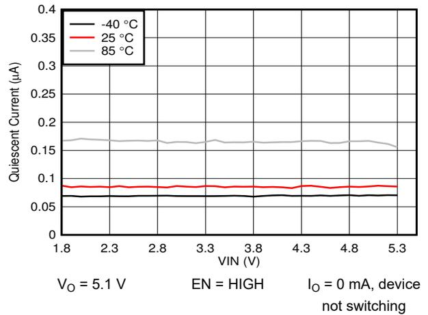
**图 6-2. Quiescent Current into VOUT versus Input Voltage**
