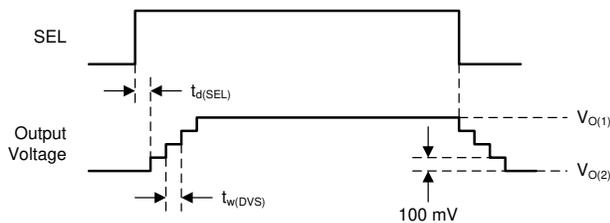
图 7-10. Dynamic Voltage Scaling with High Load
