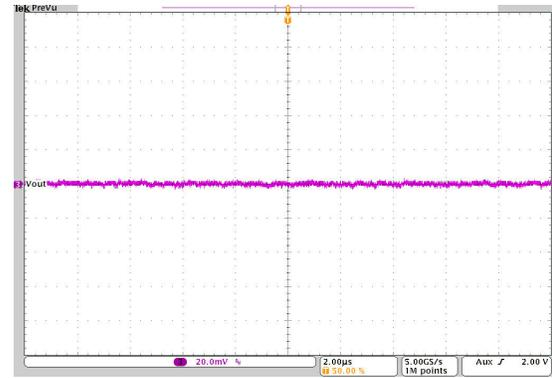
$V_{OUT} = 0.6\text{ V}$       PWM       $T_A = 25^\circ\text{C}$
