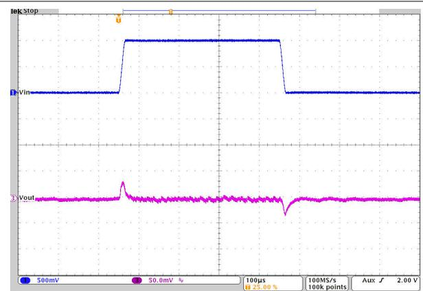
$V_{OUT} = 3.3\text{ V}$       PWM       $T_A = 25^\circ\text{C}$
