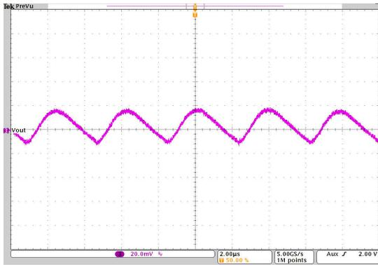
$V_{OUT} = 0.6\text{ V}$       PFM       $T_A = 25^\circ\text{C}$
