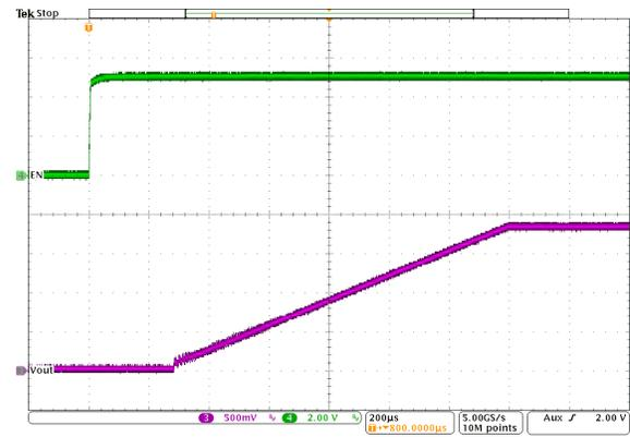
$V_{OUT} = 1.8\text{ V}$       PWM       $T_A = 25^\circ\text{C}$
