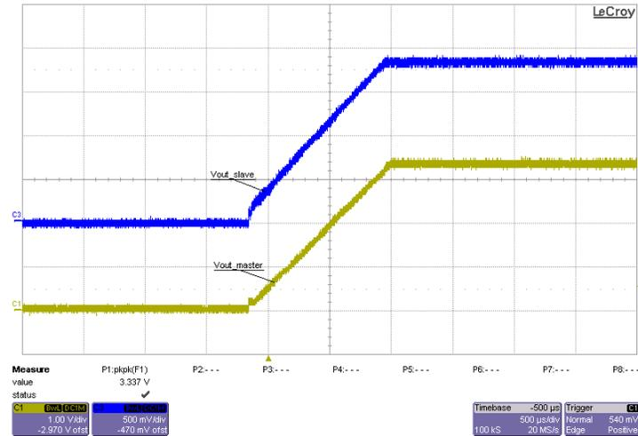
图 10-58. Scope Plot for Output Voltage Tracking
