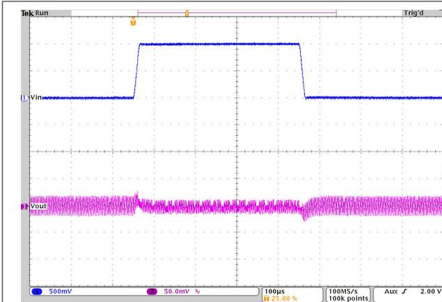
$V_{OUT} = 1.0\text{ V}$       PFM       $T_A = 25^\circ\text{C}$
