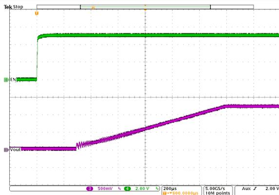
$V_{OUT} = 1.2\text{ V}$       PFM       $T_A = 25^\circ\text{C}$
