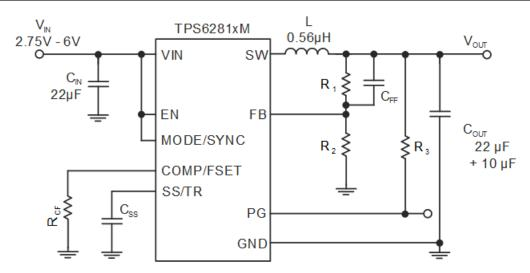
图 8-2. Measurement Setup for TPS62811M (1 A) and TPS62812M (2 A)
