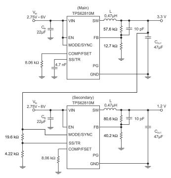
图 10-57. Schematic for Output Voltage Tracking
