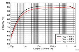
效率与输出电流间的关系; VOUT = 3.3V; PWM 和 PFM: fS = 2.25MHz
