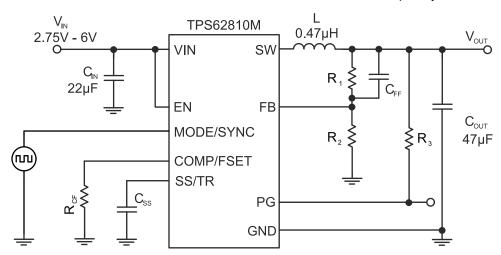
图 10-59. Schematic Using External Synchronization
