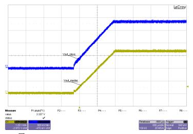
图 10-58. Scope Plot for Output Voltage Tracking
