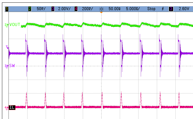
图 9-14. PFM (Power Save Mode) Mode Operation
