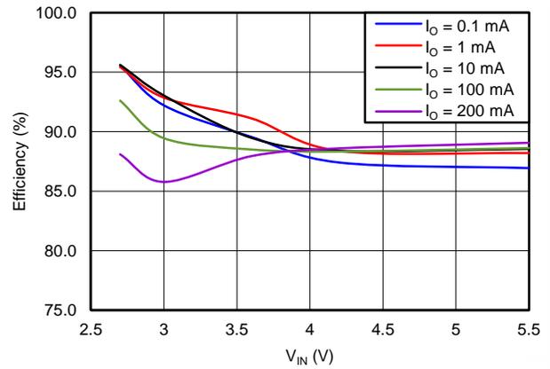
Figure 41. Efficiency vs Input Voltage,  $V_{OUT} = 2.5\text{ V}$
