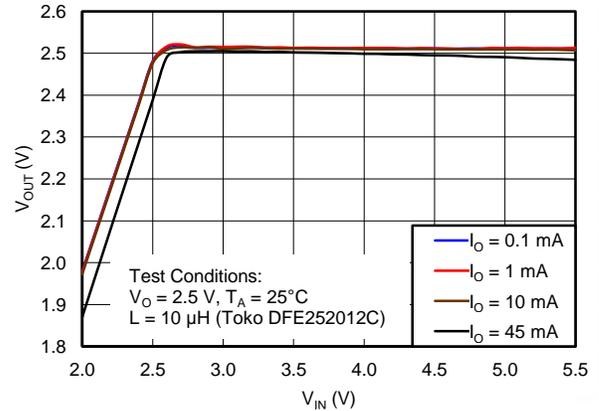
Figure 12. Output Voltage vs Input Voltage,  $V_{OUT} = 2.5$  V
