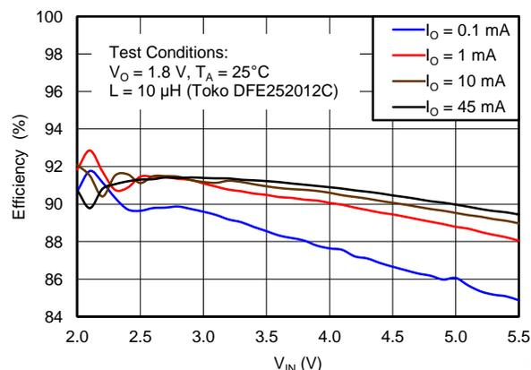
Figure 8. Efficiency vs Input Voltage,  $V_{OUT} = 1.8\text{ V}$
