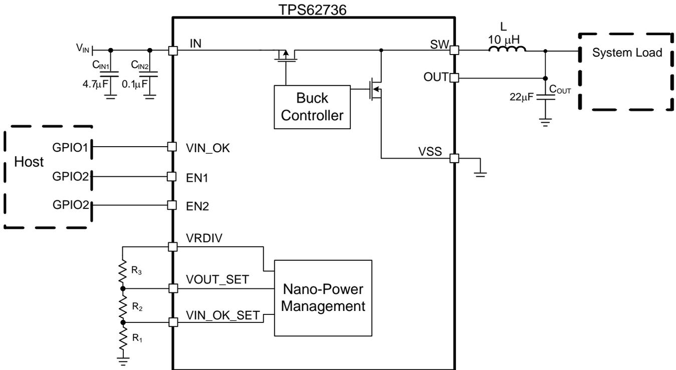
Figure 1. Typical Application Circuit for a 3-resistor String
