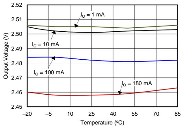
Figure 48. Output Voltage vs Temperature,  $V_{OUT} = 2.5$  V
