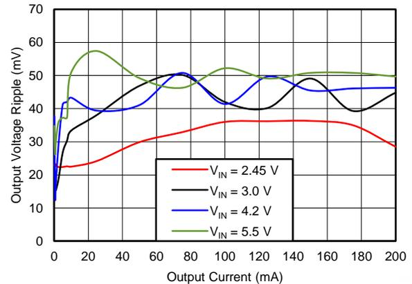
Figure 63. Output Voltage Ripple vs. Output Current
