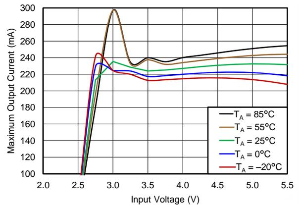
Figure 55. Maximum Output Current vs. Input Voltage,  $V_{OUT} = 2.5\text{ V}$
