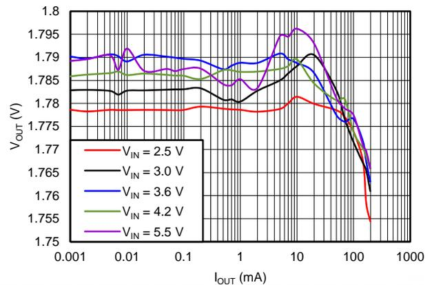
Figure 49. Output Voltage vs Output Current,  $V_{OUT} = 1.8$  V
