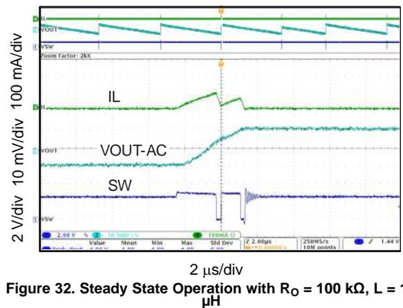
Figure 32. Steady State Operation with  $R_O = 100 \text{ k}\Omega$ ,  $L = 10 \mu\text{H}$
