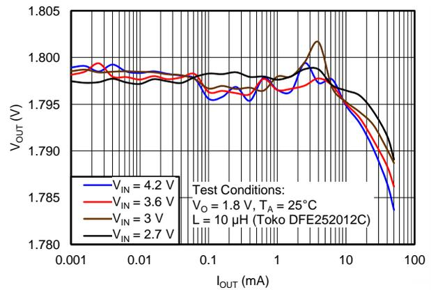
Figure 14. Output Voltage vs Output Current,  $V_{OUT} = 1.8$  V
