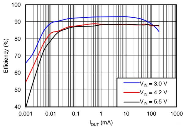
Figure 40. Efficiency Vs Output Current,  $V_{OUT} = 2.5\text{ V}$
