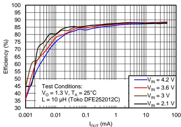
Figure 9. Efficiency Vs Output Current,  $V_{OUT} = 1.3\text{ V}$
