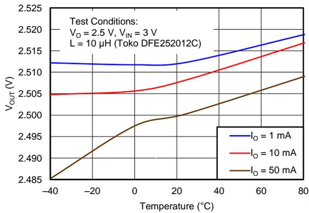
Figure 13. Output Voltage vs Temperature,  $V_{OUT} = 2.5$  V
