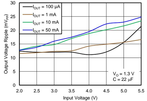
Figure 30. Output Voltage Ripple vs Input Voltage
