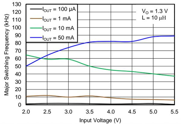
Figure 28. Major Switching Frequency vs Input Voltage
