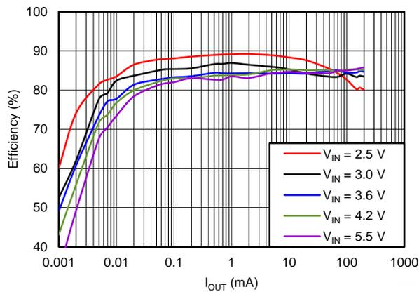
Figure 42. Efficiency Vs Output Current,  $V_{OUT} = 1.8\text{ V}$
