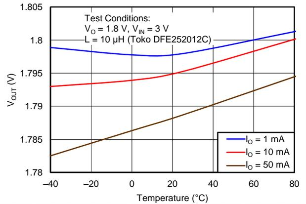
Figure 16. Output Voltage vs Temperature,  $V_{OUT} = 1.8$  V
