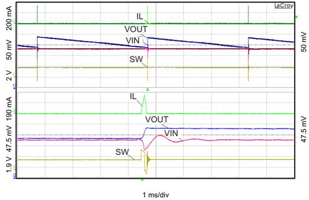
Figure 65. Steady State Operation with  $R_O = 100\text{ k}\Omega$
