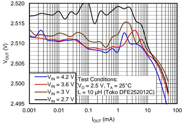
Figure 11. Output Voltage vs Output Current,  $V_{OUT} = 2.5$  V
