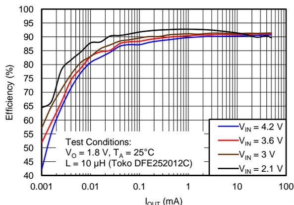
Figure 7. Efficiency Vs Output Current,  $V_{OUT} = 1.8\text{ V}$
