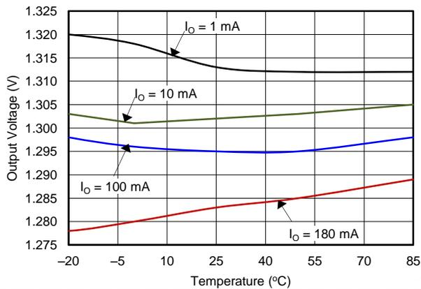
Figure 54. Output Voltage vs Temperature,  $V_{OUT} = 1.3\text{ V}$
