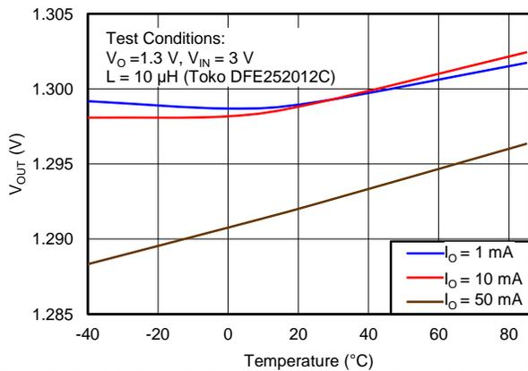
Figure 19. Output Voltage vs Temperature,  $V_{OUT} = 1.3\text{ V}$
