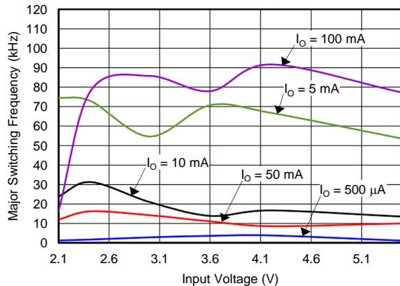
Figure 62. Major Switching Frequency vs. Input Voltage
