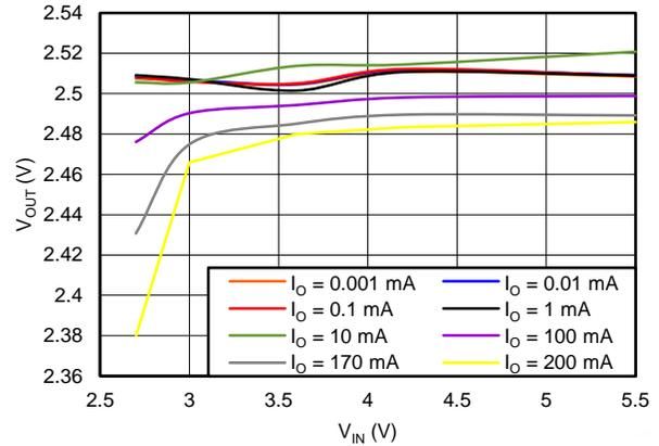
Figure 47. Output Voltage vs Input Voltage,  $V_{OUT} = 2.5$  V
