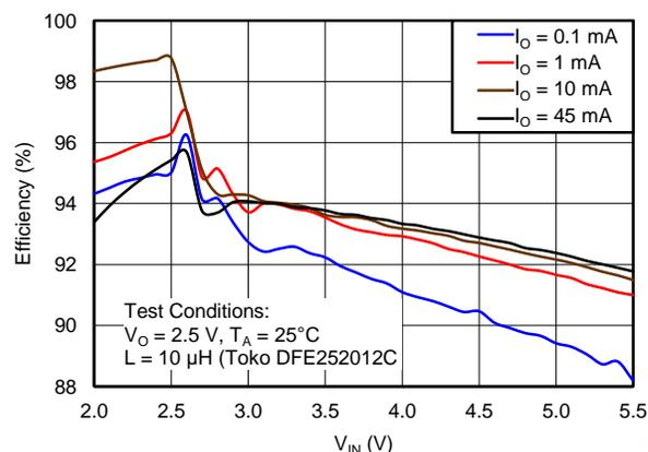
Figure 6. Efficiency vs Input Voltage,  $V_{OUT} = 2.5\text{ V}$
