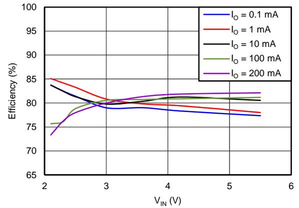
Figure 45. Efficiency vs Input Voltage,  $V_{OUT} = 1.3\text{ V}$
