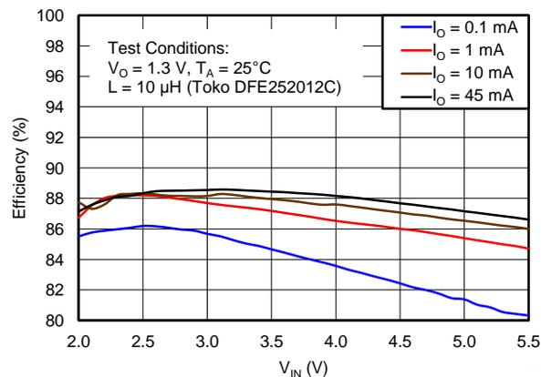
Figure 10. Efficiency vs Input Voltage,  $V_{OUT} = 1.3\text{ V}$
