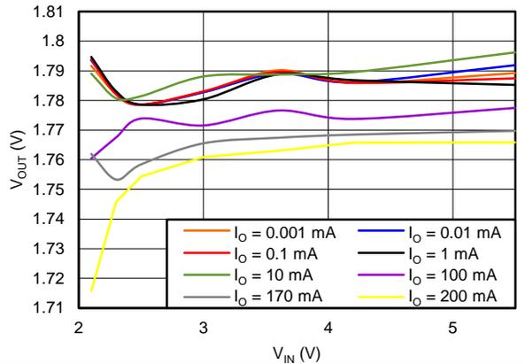
Figure 50. Output Voltage vs Input Voltage,  $V_{OUT} = 1.8$  V
