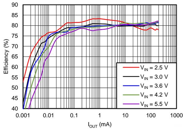
Figure 44. Efficiency Vs Output Current,  $V_{OUT} = 1.3\text{ V}$
