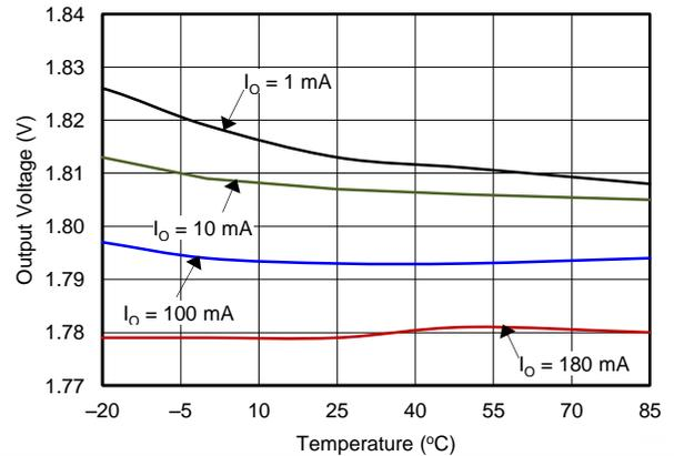
Figure 51. Output Voltage vs Temperature,  $V_{OUT} = 1.8$  V
