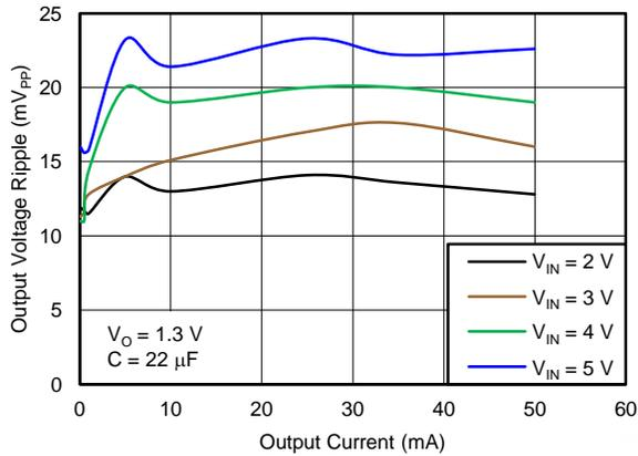
Figure 29. Output Voltage Ripple vs Output Current
