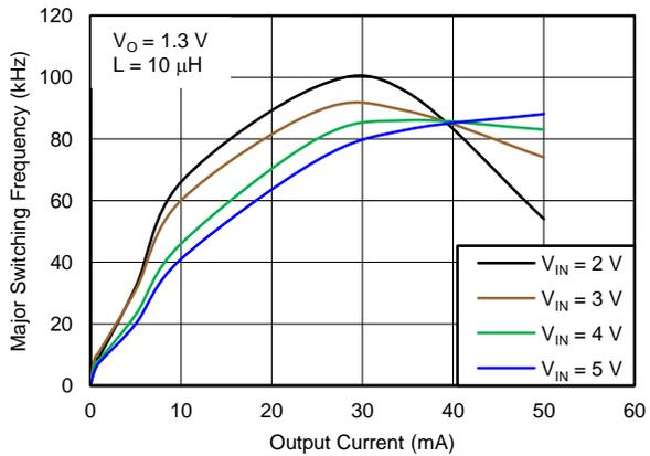
Figure 27. Major Switching Frequency vs Output Current
