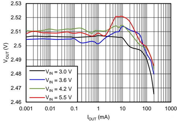
Figure 46. Output Voltage vs Output Current,  $V_{OUT} = 2.5$  V
