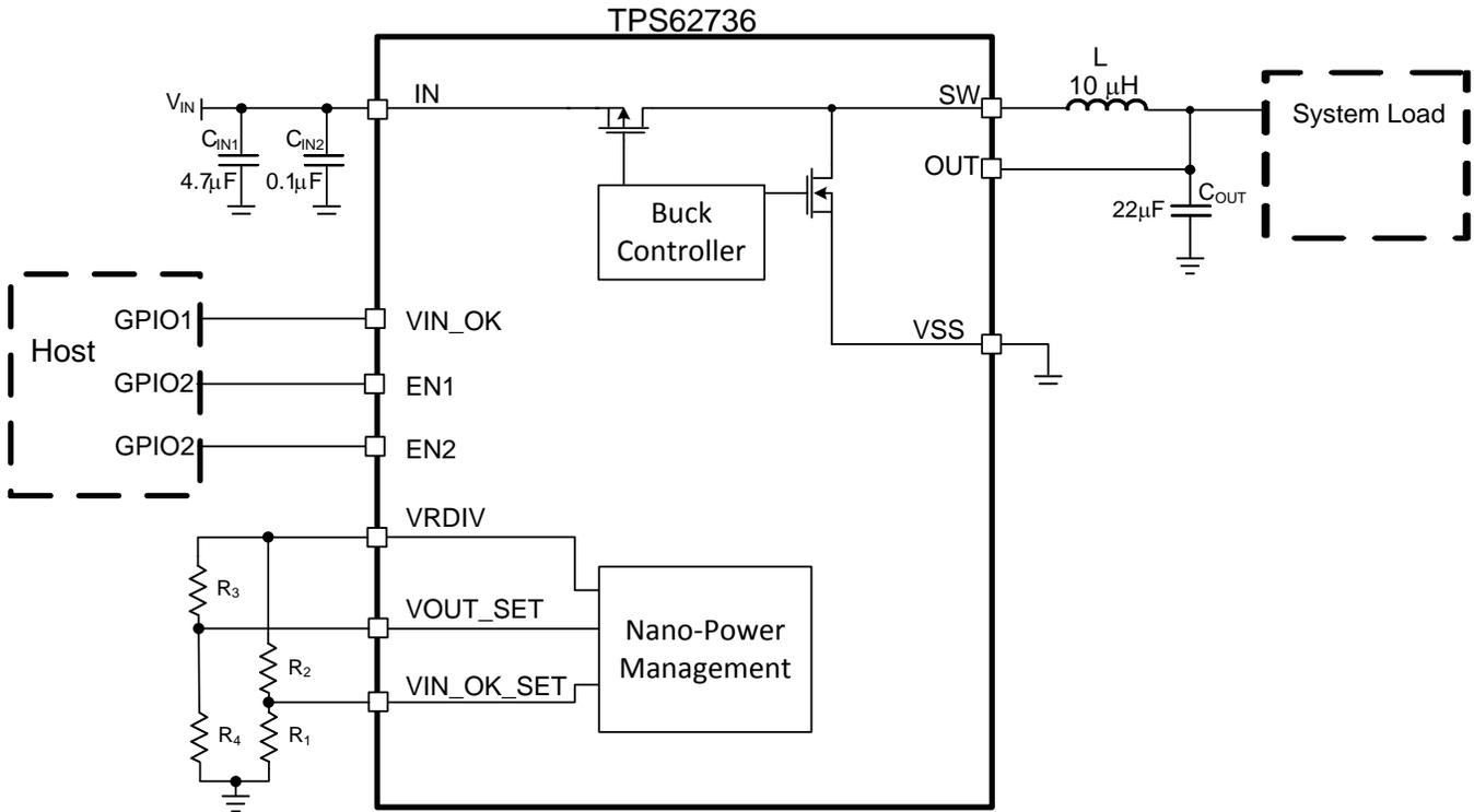
Figure 3. Typical Application Circuit for a 4-resistor String
