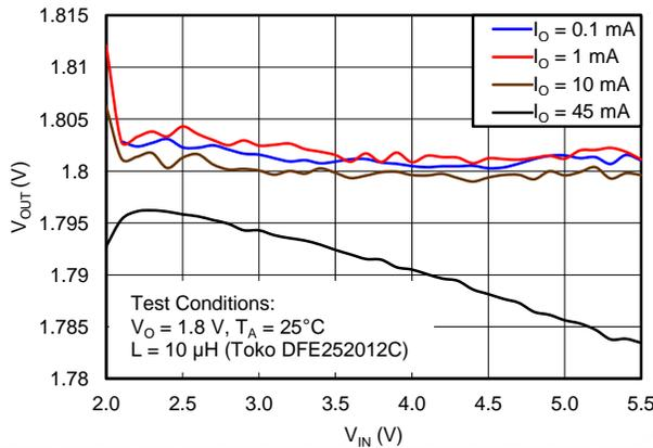
Figure 15. Output Voltage vs Input Voltage,  $V_{OUT} = 1.8$  V
