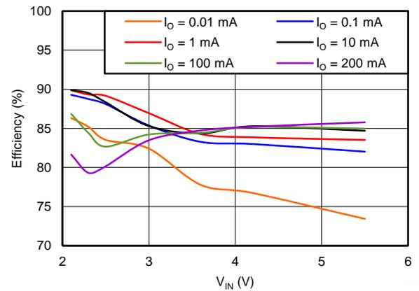
Figure 43. Efficiency vs Input Voltage,  $V_{OUT} = 1.8\text{ V}$
