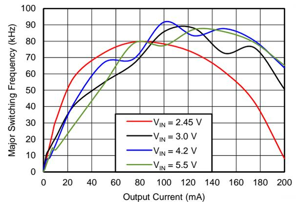
Figure 61. Major Switching Frequency vs. Output Current
