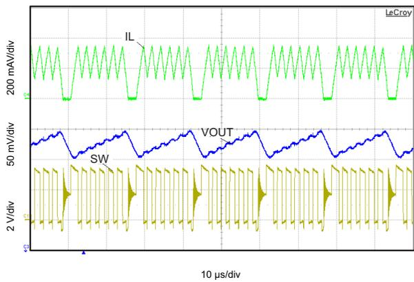
Figure 66. Steady State Operation with  $R_O = 9\ \Omega$
