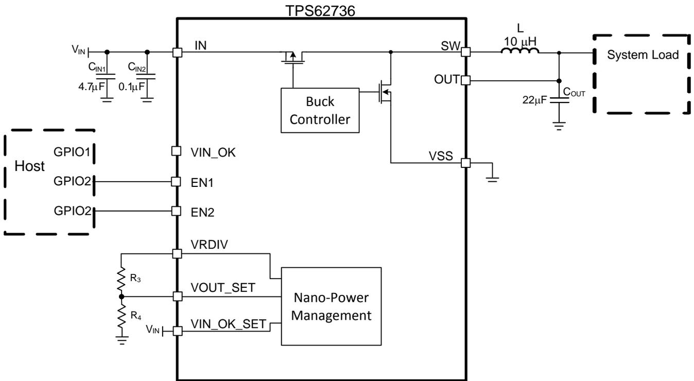
Figure 4. Typical Application Circuit for Disabling VIN\_OK
