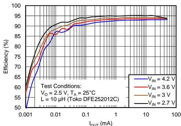
Figure 5. Efficiency Vs Output Current,  $V_{OUT} = 2.5\text{ V}$
