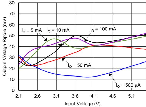
Figure 64. Output Voltage Ripple vs Input Voltage
