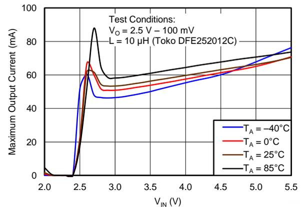
Figure 20. Maximum Output Current vs. Input Voltage,  $V_{OUT} = 2.5\text{ V}$
