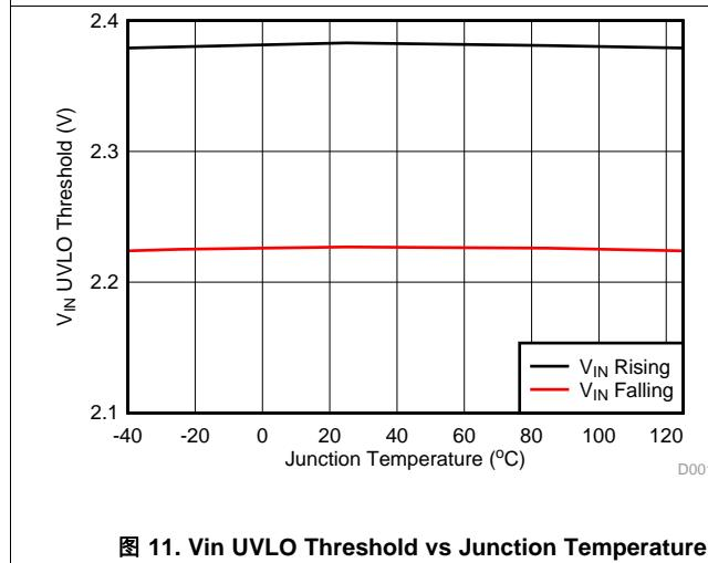
图 11.  $V_{IN}$  UVLO Threshold vs Junction Temperature
