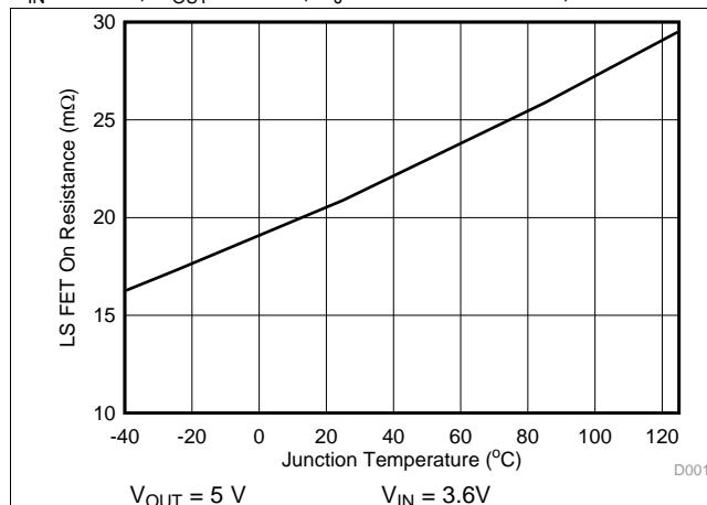
图 7. Low-Side FET  $R_{dson}$  vs Junction Temperature
