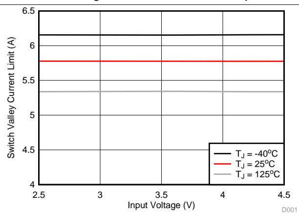
图 10. Switch Valley Current Limit vs Input Voltage
