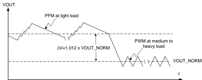
**图 14. Output Voltage in PFM / PWM Mode**
