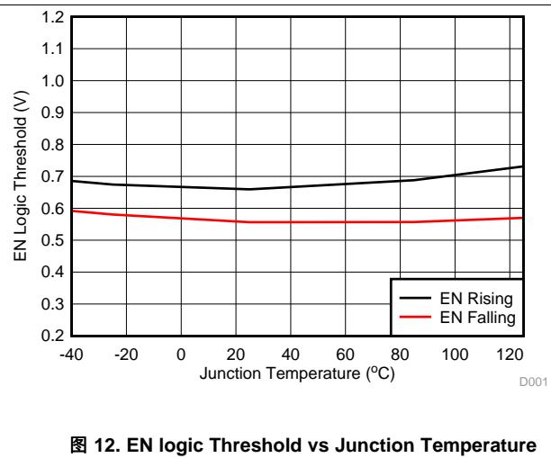
图 12. EN logic Threshold vs Junction Temperature
