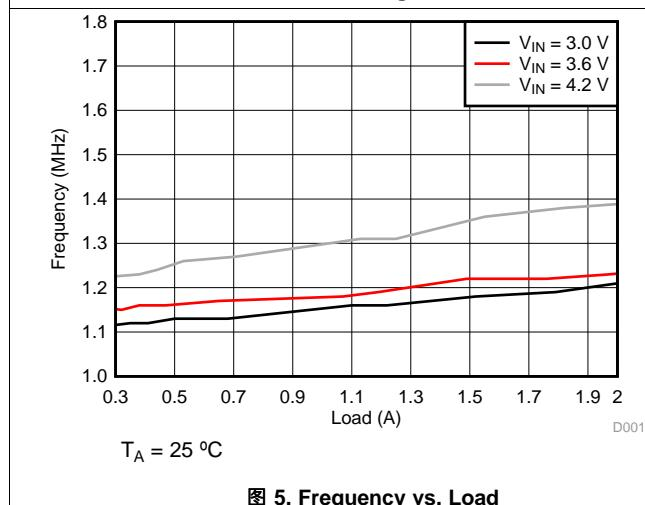
图 5. Frequency vs. Load
