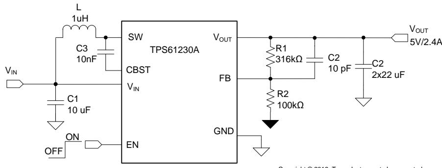
**图 25. TPS61230A 5-V Output with Cff Typical Application**
