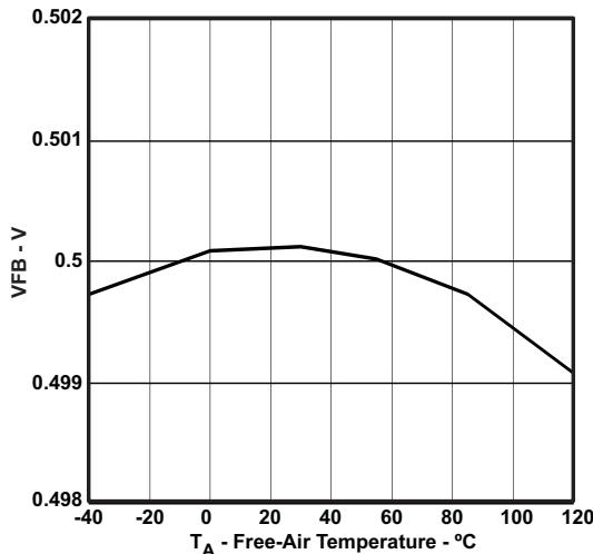
Figure 3. FB Voltage vs Free-Air Temperature
