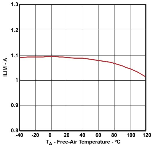
Figure 5. Switch Current Limit vs Free-Air Temperature
