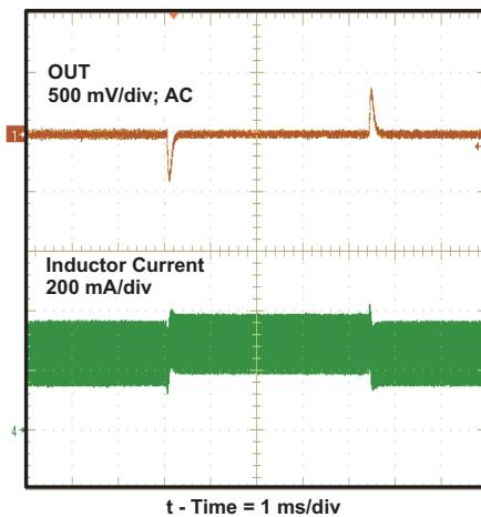
**Figure 10. 3.3 V to 3.6 V Line Transient Response**
