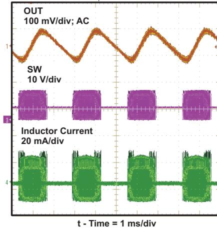
**Figure 14. Pulse Skip Mode at Light Load**
