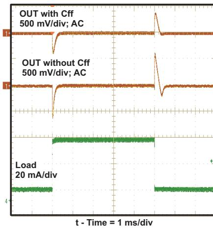
**Figure 11. 10 mA to 50 mA Load Transient Response**
