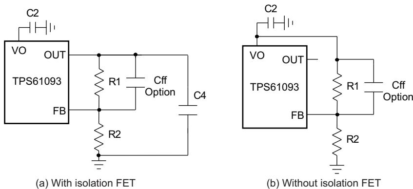
Figure 7. Resistor Divider to Program Output Voltage
