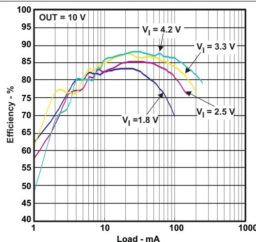
Figure 2. Efficiency vs Load
