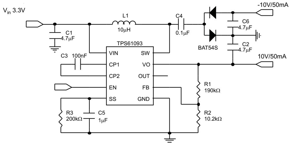
Figure 16. 10 V, -10 V Dual Output Boost Converter Schematic
