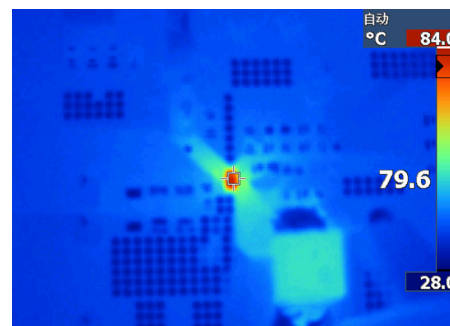
图 8-7. Case Temperature, V_{IN} = 24\text{ V} , I_{OUT} = 3\text{ A} , f_{sw} = 500\text{ kHz}
