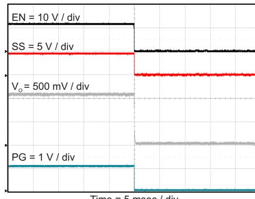
**Figure 32. TPS562210 Shut Down Relative To  $EN$**
