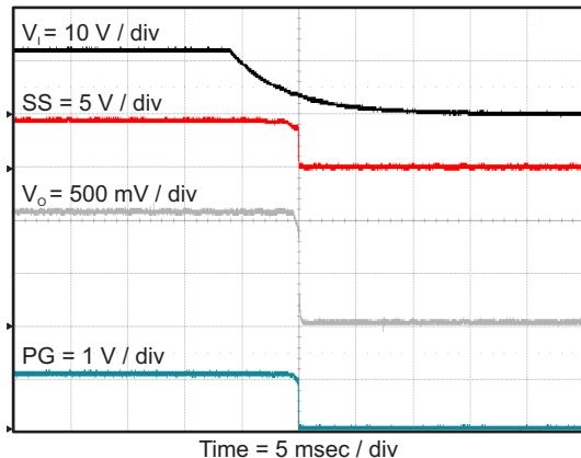
**Figure 46. TPS563210 Shut Down Relative To  $V_i$**
