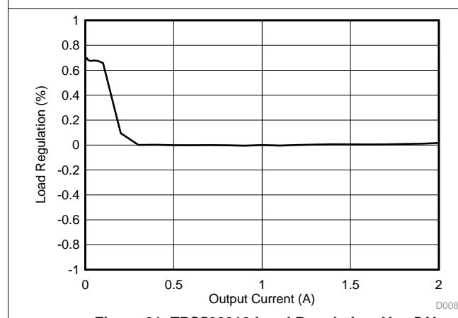
**Figure 21. TPS562210 Load Regulation,  $V_I = 5\text{ V}$**
