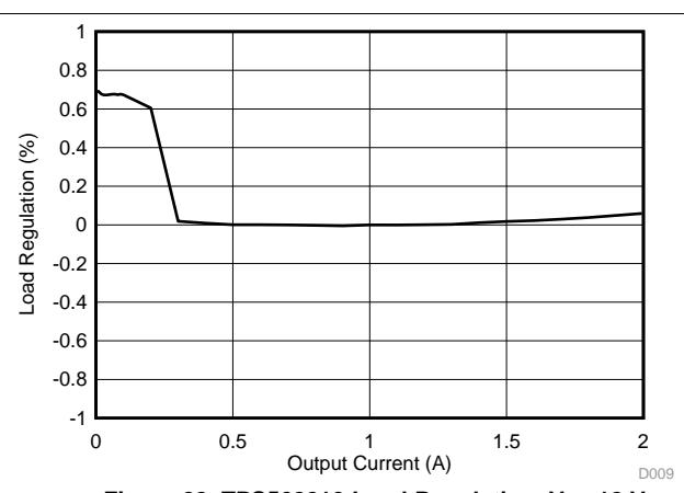
**Figure 22. TPS562210 Load Regulation,  $V_I = 12\text{ V}$**
