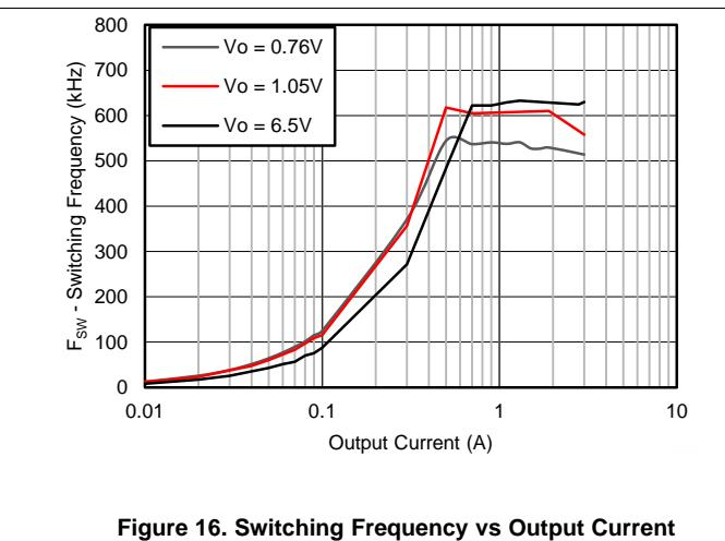
Figure 16. Switching Frequency vs Output Current
