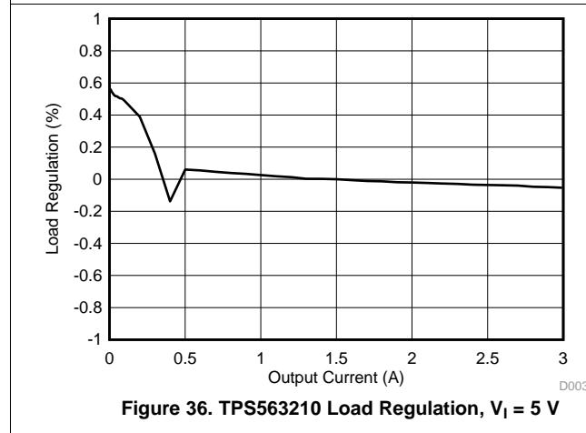
Figure 36. TPS563210 Load Regulation,  $V_1 = 5 V$
