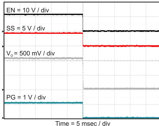
**Figure 47. TPS563210 Shut Down Relative To EN**
