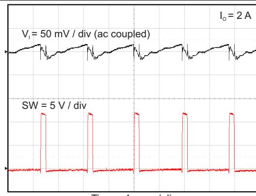
**Figure 24. TPS562210 Input Voltage Ripple**
