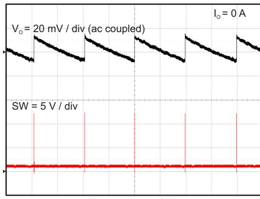
**Figure 40. TPS563210 Output Voltage Ripple**
