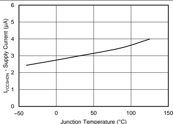
**Figure 10. VIN Shutdown Current vs Junction Temperature**
