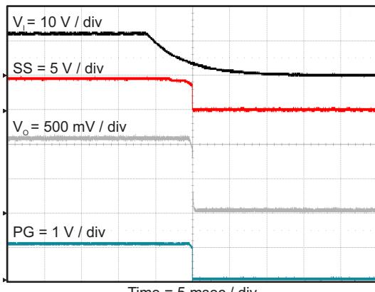
**Figure 31. TPS562210 Shut Down Relative To  $V_i$**
