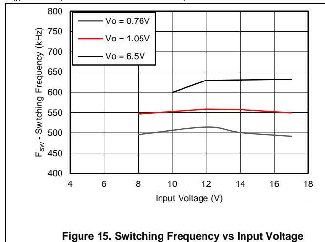
Figure 15. Switching Frequency vs Input Voltage
