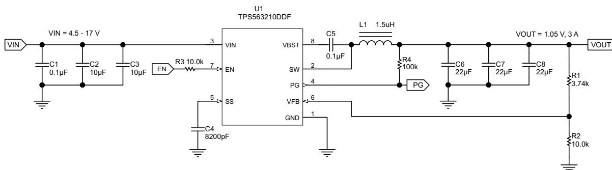
**Figure 33. TPS563210 1.05 V / 3A Reference Design**
