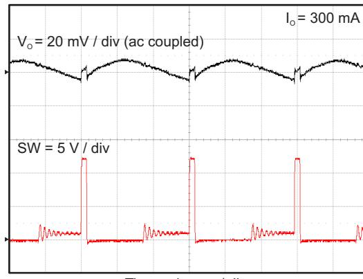
**Figure 41. TPS563210 Output Voltage Ripple**
