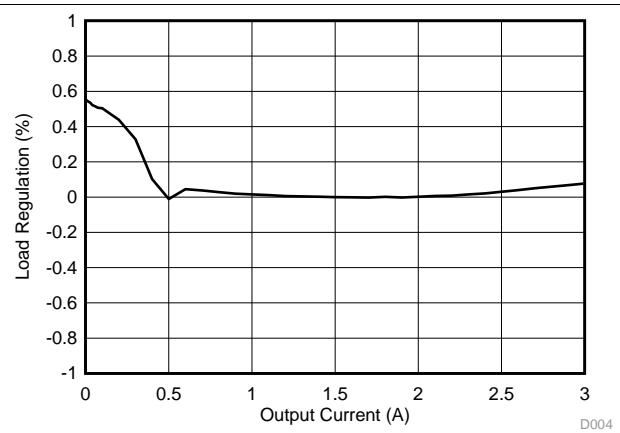
Figure 37. TPS563210 Load Regulation,  $V_1 = 12 V$
