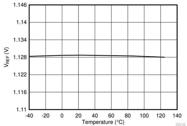
**图 6-16. Reference Voltage vs Temperature ( $V_{REF} = 1.129\text{ V}$ )**
