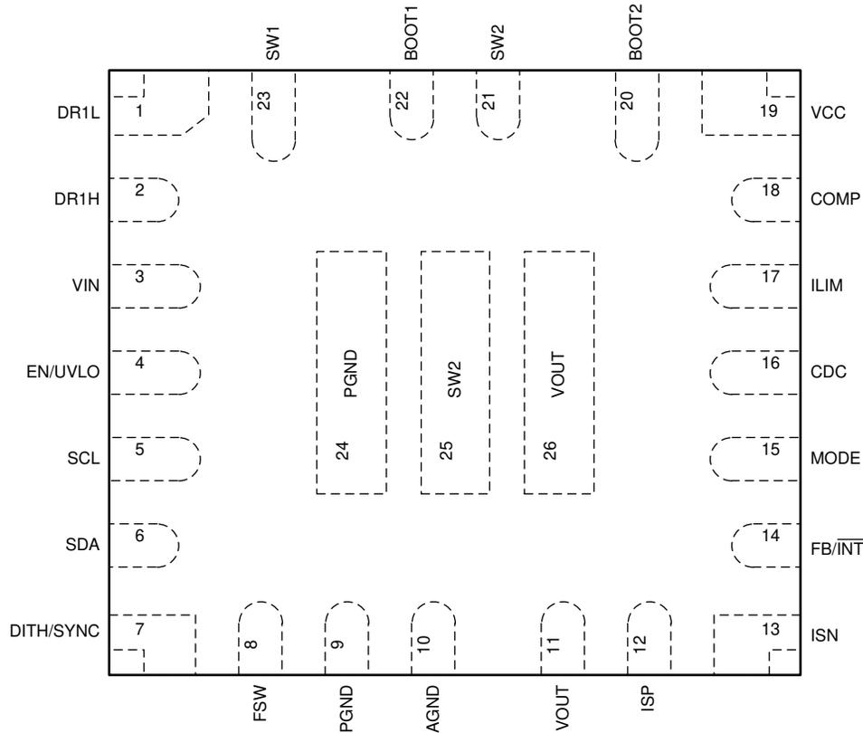
图 5-1. 26-pin VQFN-HR, RPM Package (Transparent Top View)
