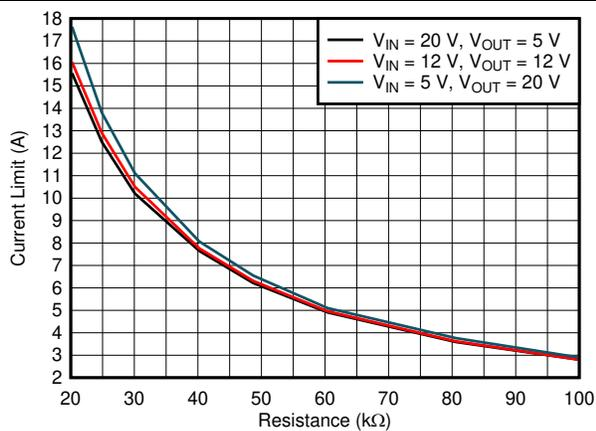
图 6-11. Average Inductor Current Limit vs Setting Resistance
