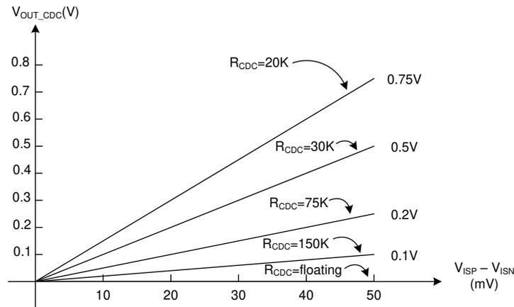
图 7-6. Output Voltage Rise versus Output Current
