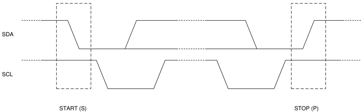
图 7-8. I<sup>2</sup>C START and STOP Conditions
