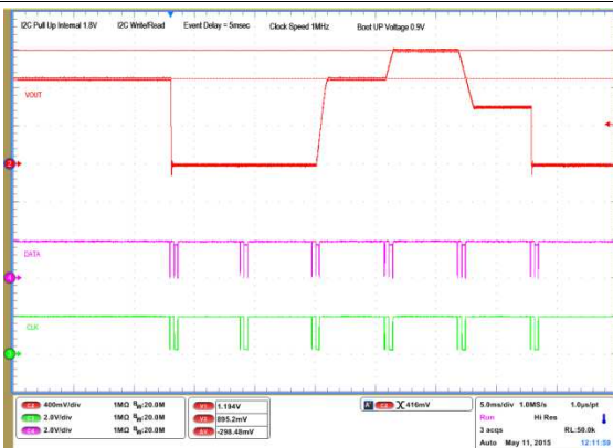
Figure 13. PMBus 1-MHz Bus Speed with 1.8-V Pullup
