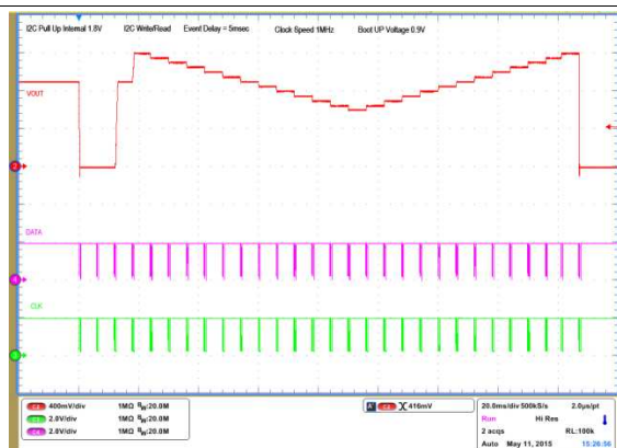
Figure 19. 17 Sequenced Events – I2C Write/Read with PEC
