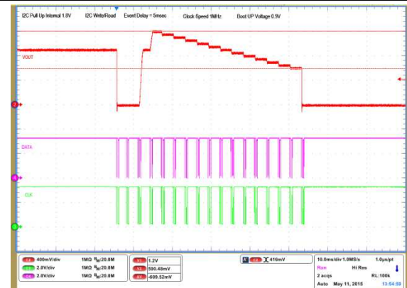
Figure 16. 6 Sequenced Events – I2C Write/Read with PEC
