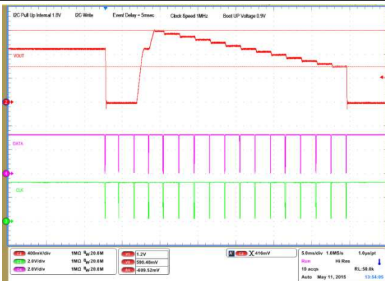
Figure 15. 6 Sequenced Events – I2C Write/Read
