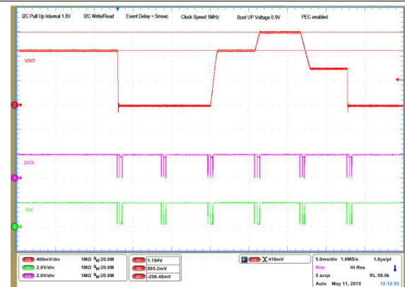
Figure 14. 6 Sequenced Events – I2C Write
