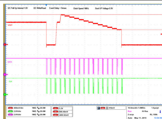
图 5-16. 6 Sequenced Events – I2C Write/Read with PEC
