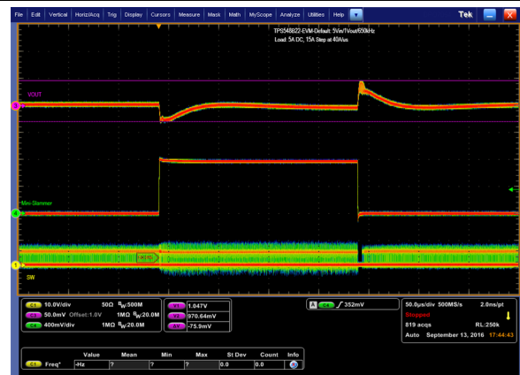
V_{DD} = V_{IN} = 5\text{ V} f_{SW} = 650\text{ kHz} FCCM Mode V_{OUT} = 1\text{ V} 5 A DC with 15-A step at 40A/ \mu s
