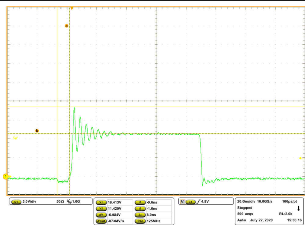
图 6-22. Switch Node Ringing and Dead-Time at 10-A Output Current
