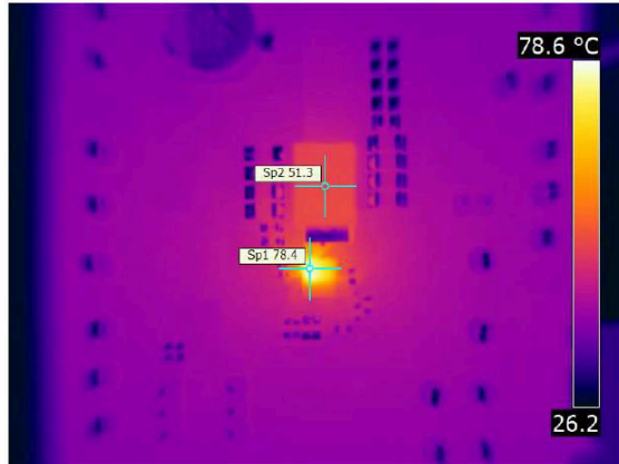
图 6-13. Thermal Image at 15-A Output Current
