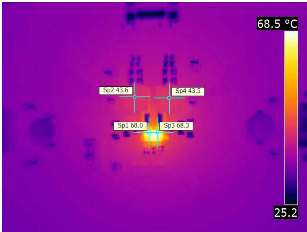
图 10-3. Thermal Image at 25°C Ambient - 2-phase Operation, f_{sw} = 1\text{ MHz} , V_{IN} = 12\text{ V} , V_{OUT} = 1\text{ V} , I_{OUT} = 12\text{ A} , Inductor = 560 nH (3.3 m \Omega typical)
