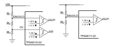
图 8-12. Programming Overvoltage and Undervoltage Protection Threshold
