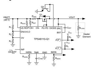
图 9-1. Typical Application Schematic: Driving HVAC PTC Heater
