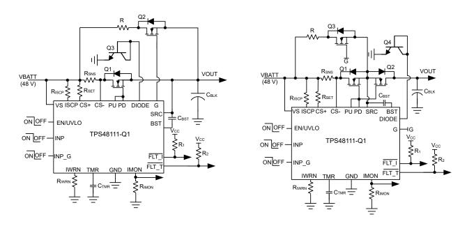
图 8-8. TPS48111-Q1 application Circuits for Capacitive Load Driving Using Precharge FET and a Series **Power Resistor**
