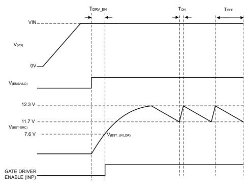
图 8-4. Charge Pump Operation
