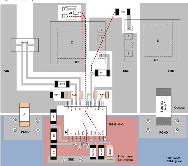
图 9-19. Typical PCB Layout Example With TPS48110-Q1 With B2B MOSFETs
