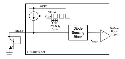
图 8-13. DIODE based Remote Temperature Sensing Block Diagram
