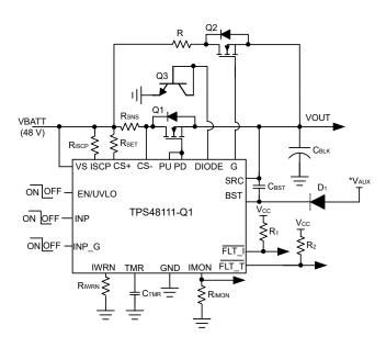
图 8-5. TPS48111-Q1 Application Circuit with external supply to BST
