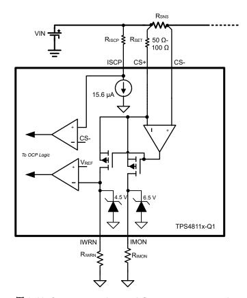
图 8-11. Current sensing and Overcurrent protection
