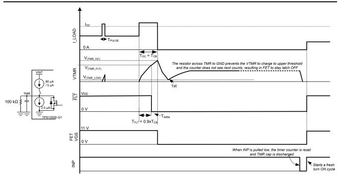
图 8-10. Overcurrent Protection With Latch-Off
